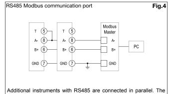
serial output must only be terminated on the last network device connecting terminals B+ and T. For connections longer than 1000 m or networks with more than 160 instruments, use a signal repeater.
