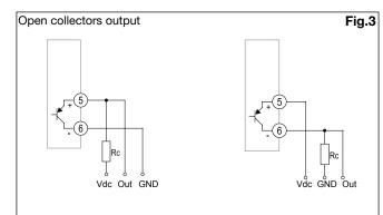
The load resistance (Rc) must be designed so that the closed contact current is under 100 mA ( $V_{on}$  is equal to 1 V dc). DC voltage ( $V_{off}$ ) must be less than or equal to 80 V.
