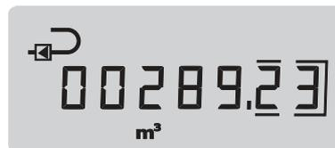
Basically accumulated energy is displayed. Activating the push-button the display immediately switches to other readings. The display automatically returns to energy reading four minutes after the latest activation of the push-button, and after four more minutes without activation the display switches off in order to save current.
