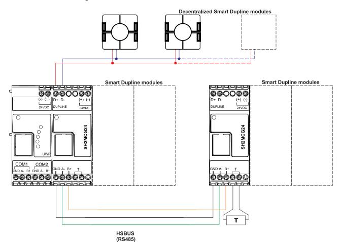
Fig. 3 Example of Smart Dupline modules connection using master channel generators
