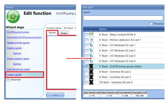
The signals available in this window are LEDs and relays.
