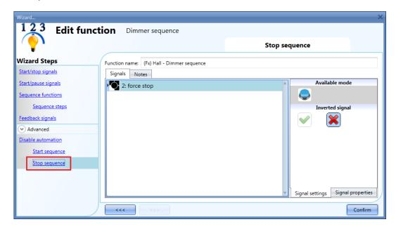
Each signal used in the *Stop sequence* window works in level mode. While the *Stop signal* is active, the function is stopped and cannot be activated until the stop signal disappears.
