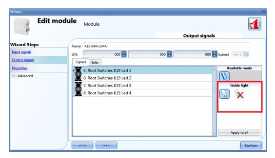
In the *Output signals* window, the user can enable the white LED as a guide light (red rectangle): by clicking on the white LED icon, the guide light is enabled, while by clicking on the red cross the guide light is not enabled.
