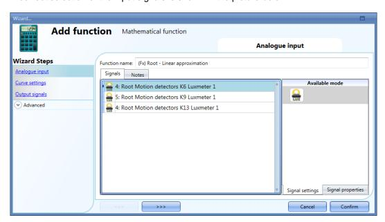
All the added signals are of the same type (three lux-meters).
