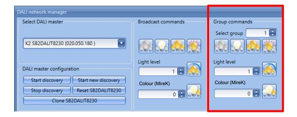
To test the ballasts that belong to a specific DALI group, the user has to enter the group number (from 1 to 16) in the *Select group* text-box and press on one of the commands available.
