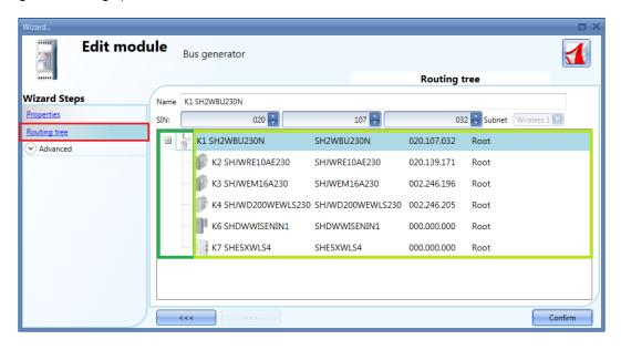
Example 2: SHDWWISENIN1 and SHE5XWLS4 modules are connected indirectly and they use the SHJWD200WEWLS230 module as a router to communicate with the wireless base unit (see the green rectangle in the picture below). The SHJWRE10AE230 and the SHJWEM16AE230 are directly connected to the wireless base unit.
