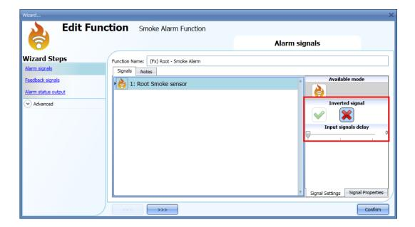
To add the alarm output, the user should select the relevant section in the wizard of the function, then double click on the *Signals* window and select the input signal from the list of those available (see picture below).
