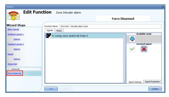
Each signal used in the *Force alarm disarmed* window works as a level signal. Until the signal is active, the main alarm function, and all linked zones, are forced into disarmed.
