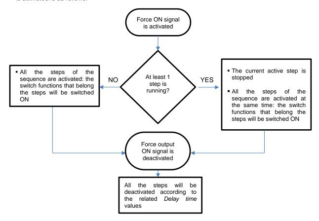
NOTE: When the Force output fully on signal is activated and at the same time the Force output fully off signal is activated, the Signal Off has priority and the Force output fully off command is executed.
