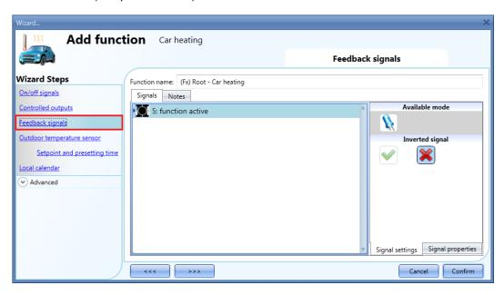
The feedback signal can be a relay, a LED or a buzzer, and it follows the status of the function: when the function is ON the feedback is on, when the function is OFF the feedback is off.
