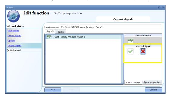
The inverted logic for the output signals can be selected in the *Signal settings* tab window, as shown in the yellow rectangle above.
