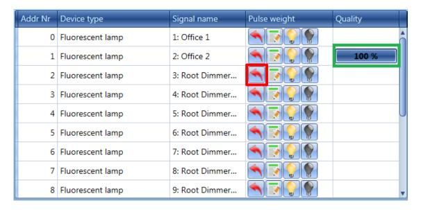
By means of the *Reset* button, the user can bring the ballast back to the factory settings. This means that should this ballast be connected to a DALI bus, it will be recognized as a new one.
