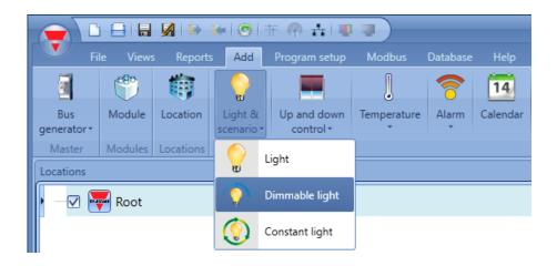
This function manages one or more dimmer outputs controlled by one or more input commands. The command might be a real signal such as a pushbutton, a function or a remote command (Webserver, sms, email, Modbus TCP/IP)
