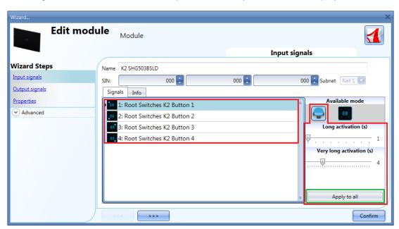
In the *Input signals* field, each key can be used in 2 different ways: as a **Push button** or as a **Dimmer Interface**.
