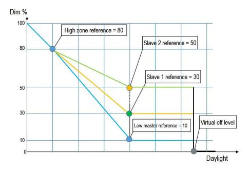
In this case the slave zones will never reach the minimum dimming level.
