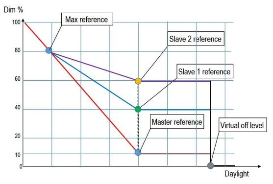
To summarize, the calibration of the master zone is needed to create its dimming curve (red line), while the calibration of the slaves zones is needed to create their dimming curve (blue and purple lines).
