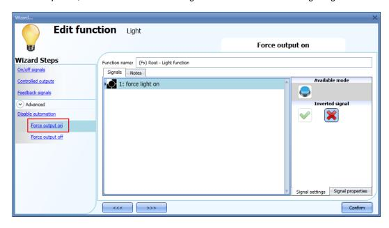
Each signal used in the *Force output on* window works as a level signal: until the signal is active, the light function is forced on.
