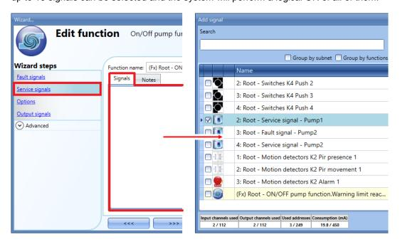
Each signal used in the *Service signals* window works as a level signal: until the signal is active, the function is forced into the OFF condition. In the *Signal settings* window the user can set the actions that have to be performed according to the different actions allowed by the system, as shown in the green rectangle below:
