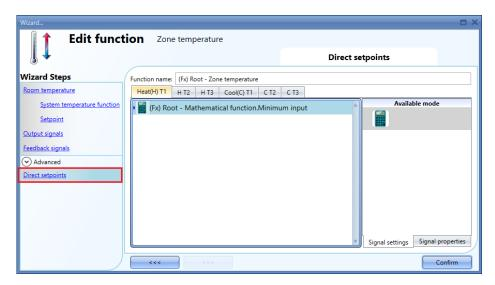
As shown in the picture above, a *Mathematical* function can be used as Heating Setpoint 1(T1) regulation, setpoint2 or setpoint3.
