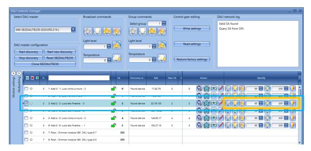
The related ballast receives the command that changes its status according to the command that has been executed by the user.
