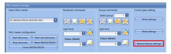
The ballast will be restored to Factory settings: this means all the settings saved in the device will be lost.
