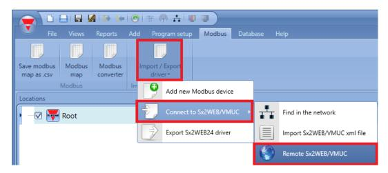
After clicking on *Remote UWP 3.0/VMUC*, the *Import manager* window will appear: insert the IP address of the remote slave device and click on *Import:* If the IP address of a remote device is not correct, the UWP 3.0 tool will prompt the following message in the *Log* window:
