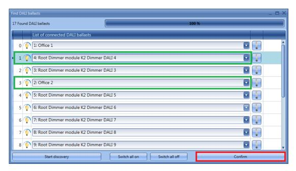
The user may move all the desired devices to the new addresses. When all the devices have been addressed, press the *Confirm* button to save the configuration.
