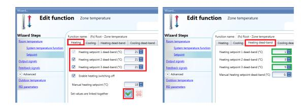
In this situation, if setpoint1 is selected, the regulating level is 20° (i.e 21-1), if setpoint2 is selected, the regulating level is 18° (i.e 21-3), if setpoint3 is selected, the regulating level is 16° (i.e 21-5). In the TEMDIS and webserver all the three setpoints will be 21°, and the changing of any one of them will also change the other two.
