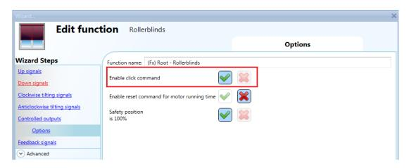
2) A **very** long press (> 0,5 sec) activates the motor output until the input signal is ON (the blind is tilted clockwise/anticlockwise until the user keeps the pushbutton pressed or the selected signal is active). This functionality doesn't need to be enabled.
