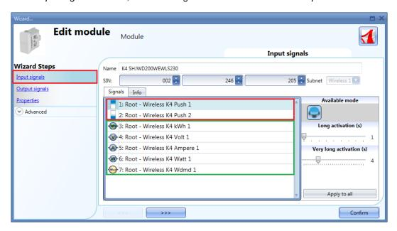
The SHJWD200WExLS230 module integrates two programmable capacitive push-buttons and can be used in all the UWP 3.0 tool functions, as shown in the red rectangle in the picture above.
