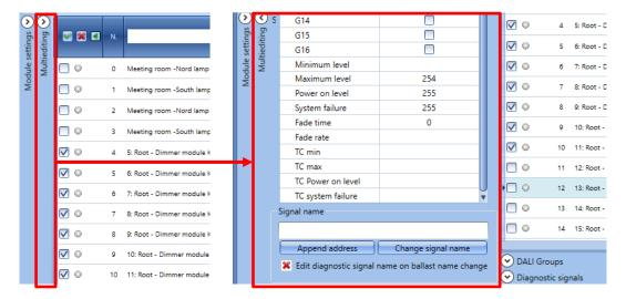
In the *Multiediting* panel, in the *Signal name* text-box, the user can type the name they want to assign to all the signals that have been selected.
