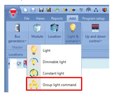
This function manages the ON/OFF switching of one or more light functions by means of one or more Group commands. The Group command might be a real signal, a function or a remote command (Webserver, Modbus TCP/IP).
