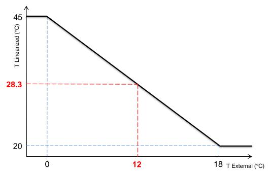
The linearized values are used as Virtual Range for the Output Range (in Volts).
