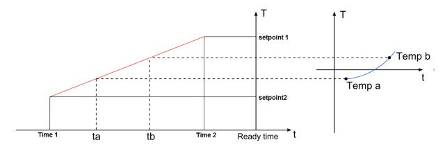
If the measured temperature has a value Temp b (higher than Temp a), the output will be activated later (at time tb), because the temperature is higher and the output requires less heating time to warm the car.
