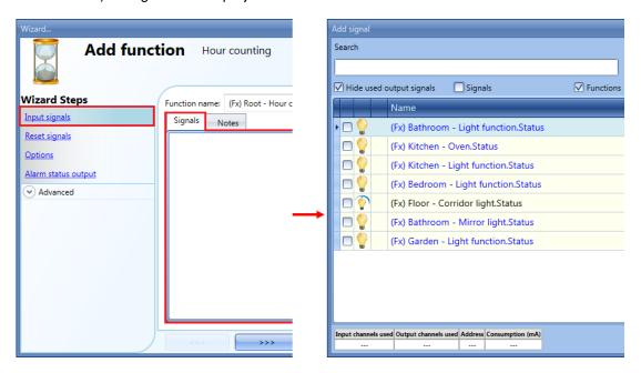
Only one input signal can be added to the Hour counting function.
