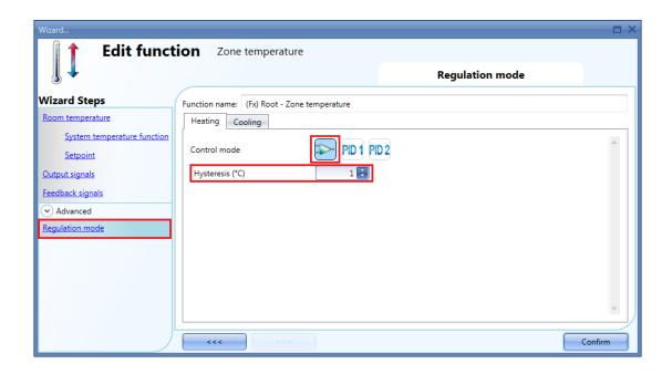
If the setpoint is 20° and the hysteresis is 1°, the output is switched off at 20° and activated again at 19°. (see the graph below)
