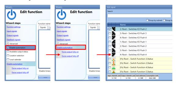
The required signal has to be added by double clicking in the Signals window.
