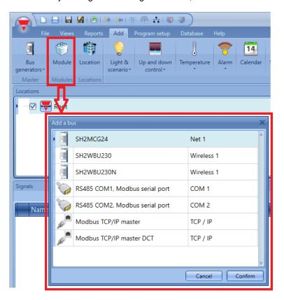
Each added SH2MCG24 will be assigned to a **new sub-network**, up to 7 Master generators/wireless Master generators.
