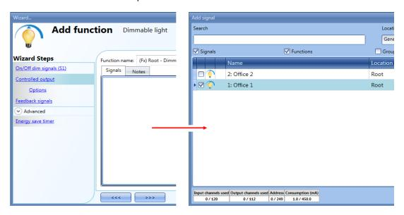
To select the output signal that is controlled by the dimmable light function, click on *Controlled output* and then double click on the *Signals* window. Once the output window is opened, select the relevant outputs from the list: up to 100 dimmer outputs can be added.
