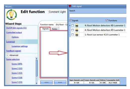
The user can add up to ten lux sensors: if more lux signals are linked to the function, the average lux value is calculated and then used.
