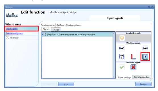
In the *Working mode* field of the Signals setting window, the *Every change* mode is selected (see the red rectangle above): whenever the *Zone temperature.Heating setpoint* signal changes, the Modbus TCP command will be sent to the Modbus device.
