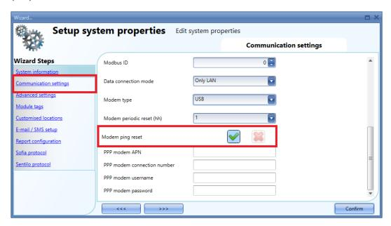
The use of the *Modem periodic reset (hh)* and/or the *Modem ping reset* options depends on the functions the user has configured in the project. There are different possible scenarios, so please consider the following recommendations:
