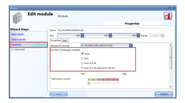
In the *Transmission power* field, the user can also manage also the transmission power of the module by moving the slider. This field is not available for the SHDWRE16AE230 module.
