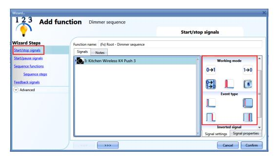
The input signal can be used either to start and/or to stop the sequence.
