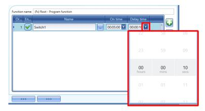
N.B: If the *Delay time* value is set to 00:00:00, the next step is activated with no delay from the previous step.
