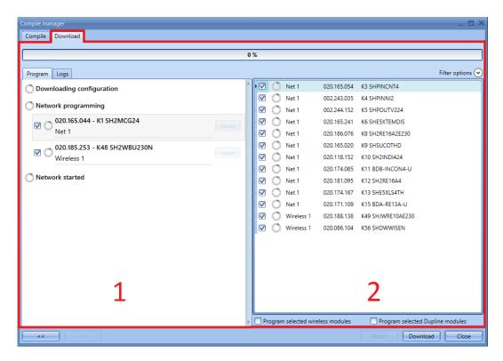
On the left side of the *Download configuration* window (**Area1**) all the networks are listed, while on the right side (**Area2**), all the modules are shown. Each module is presented with the following information: network it is connected to, SIN number and the name.
