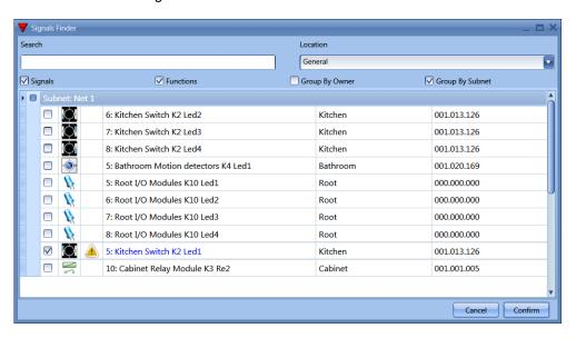
The signals available in this windows are LEDs and relays. Up to 50 signals can be chosen and they are managed in parallel.
