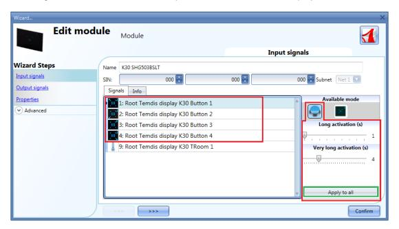
In the *Input signals* field, each key can be used in 2 different ways: as a **Push button** or as a **Temdis interface.**
