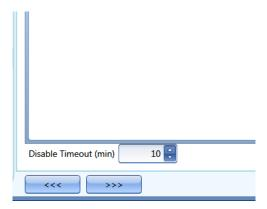
In the figure above, a disable timeout of 10 minutes is set. The maximum delay is 59 minutes.
