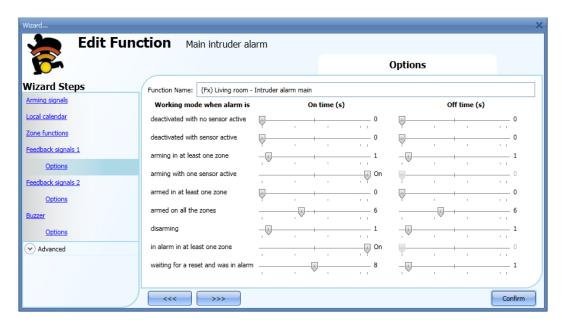
For all the statuses, the user can set the On/Off activation time. If both the on/off times are set to 0 seconds, the status will not be shown by the feedback signal.
