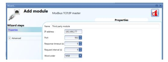
IP address: enter the address of the slave device
