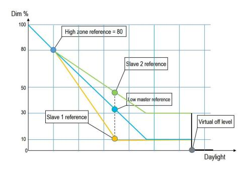
If a slave zone is nearer to the window than the master zone, its dimming curve will be below the master one and it will reach the minimum dimming value.
