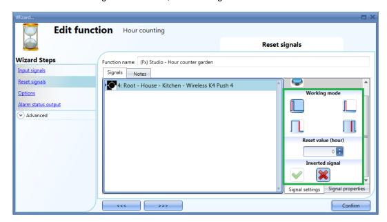
For each signal it is possible to set a certain reset value when the reset signal is triggered (e.g. when the push button is pressed): the user may set the *Reset value (hour)* field.
