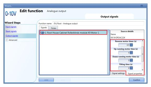
N.B The user must set the *Up running motor time* and *Down running motor time* for the Reset command: any value set in *Tilting time* will not be used.
