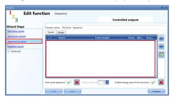
Auto cycle sequence: if this option is enabled, the sequence is repeated continuously: each time the last function is executed, the sequence starts again from the beginning. All the functions are executed in a loop and the sequence can be stopped by using the stop signal(s).
