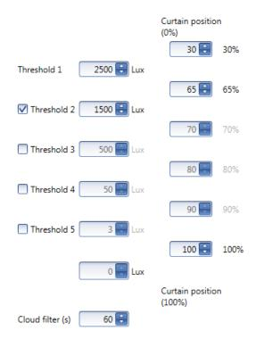
In the picture below, the behaviour of the output is shown according to the light level.
