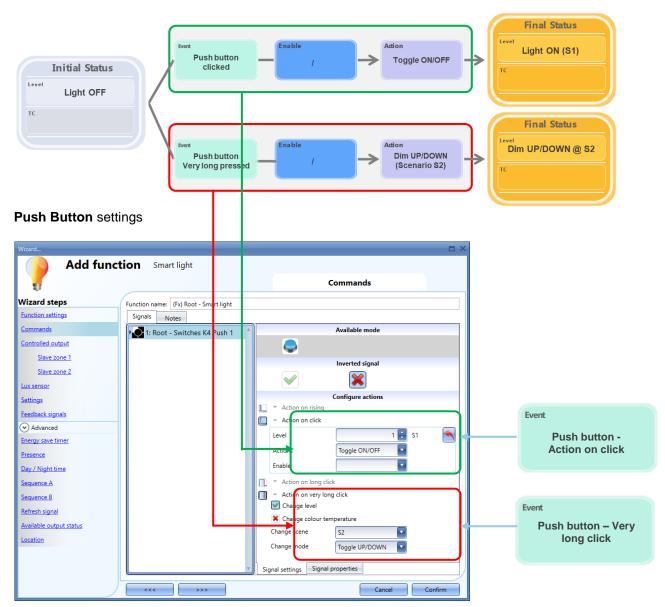
Note: you cannot select to toggle ON(S1)/OFF using Rising Edge because dimming will not work. The very long time has to be adjusted in order to speed up the dimming.
