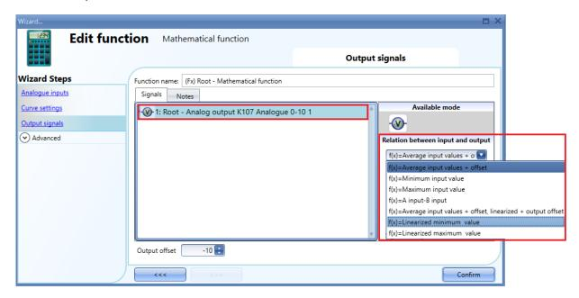
The 0-10 V output value is calculated based on a linear relation between the input and output values of the *Mathematical function*.
