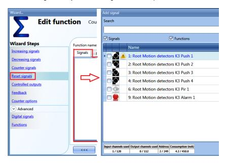
Each time the reset signal is activated, the counting value is reset.
