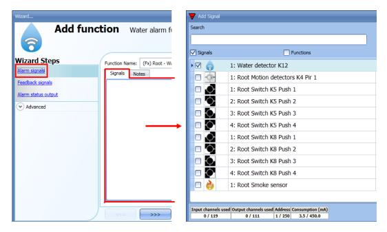
Once the alarm signal is entered, the user can also decide to use the inverted logic of the signal (see the red rectangle in the picture below). The inverted logic is enabled by selecting the green V. Each alarm signal added to the function has a delay time that can be set in order to filter the activation of the alarm when the water is detected. This may be used to avoid false alarm triggering.
