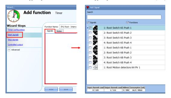
When the trigger signal is entered, the user can set the working mode, the event type and the logic for the trigger signal (shown in the picture below).
