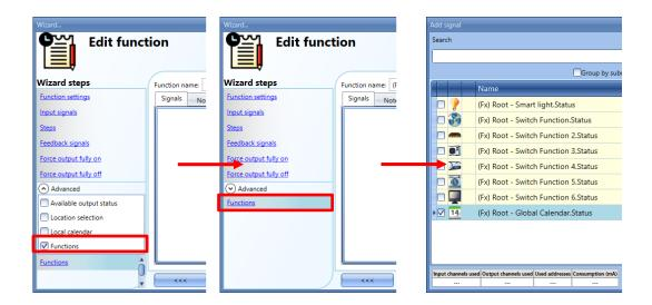
All the added functions will trigger the sequence according to their status: for example, if a *Global calendar* is added in this field it works in the same way as the internal calendar.
