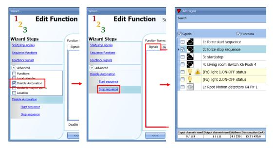
Each signal used in the *Stop sequence* window works in level mode. While the *Stop signal* is active, the function is stopped and cannot be activated until the stop signal disappears.
