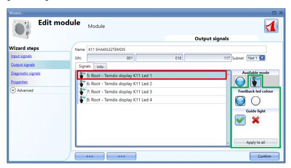
In the *Led colour* field the user can set the colour of the LED for the feedback when a push button is pressed:
