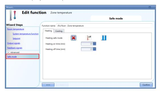
The user can then select the action to be performed when the safe condition is needed (faulty temperature sensor). In the table below the list of available actions is shown.
