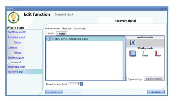
A typical application is using a BDA-INVOL-U signal inside a timer function in order to send the update command few seconds after the Power line is restored. In this way the DALI ballasts have time to start-up, as shown in the example in the example below:
