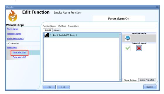
The signal used in the *Force alarm On* window works as a level signal: while the signal is active, the function is forced to the ON condition (the output stays active).
