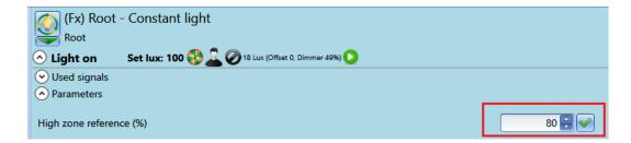
This gives the high point in calculating the dimming curve of the slave zones.
