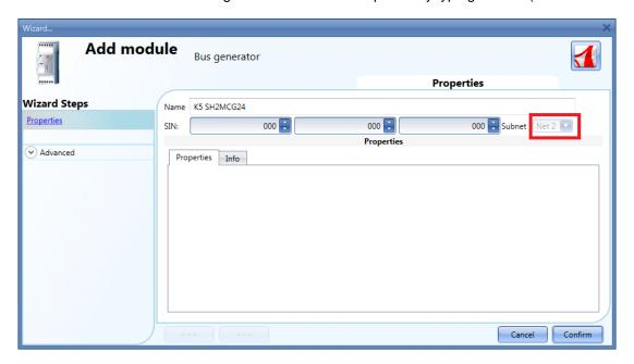
In the picture above, a new module is inserted with its associated new network (e.g. Net 2) As shown, each new generator will be assigned to the next free network (e.g. Net 2)
