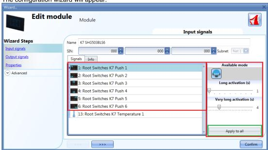
In the Input signals field, the Long activation and the Very long activation time has to be defined.
