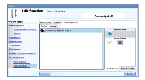
Each signal used in the *Force output off* window works as a level signal. Until the signal is active, the heating/cooling output is forced off.
