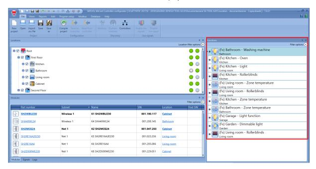
When a new function is created by the user, it will be added into this area; to edit a function already made, the user has to click on the picture of the function, the wizard will be opened.
