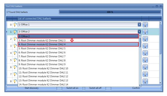
In the picture above, the ballast with address 1 (Office 2) has been addressed with address 3 (Dimmer output DALI 4)
