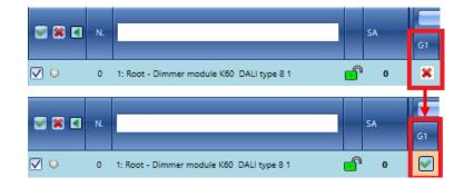
To remove the ballast from a group (1 to 16), the red X icon must be checked
