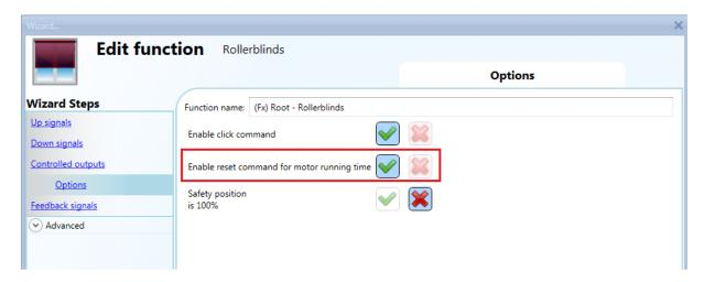
The reset command is also available via the webserver (when accessed as administrator) and via the UWP 3.0 Tool in the live signals mode. When the command is sent by using the webserver or the Tool, a window with a warning message is shown to advise the user not to stop it.
