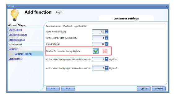
If for any reason the PIR sensor is enabled to switch the light ON also during day time, the red X in the red rectangle should be checked.
