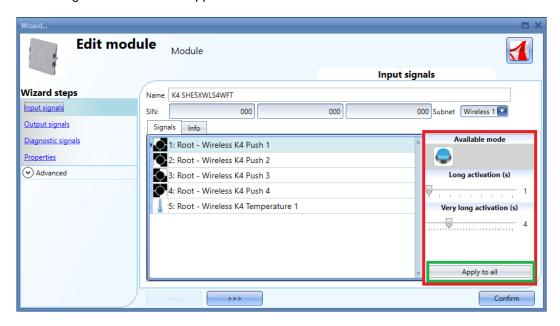
In the *Input signals* field, the *Long activation* and the *Very long* activation time has to be defined. The *Long activation* time can be set from 1 to 5 seconds, while the *Very long activation* time can be set from 0.5 to 15 seconds and it is always set by the system 3 seconds longer than the *Long activation* time. The user can configure different times for each push button, or can set them to the same values by clicking on *Apply to all*.
