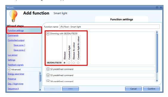
In *the Function settings* tab of the window, the user has to select the type of lighting control he needs to set. The available control types are the following ones:
