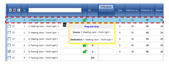
With the left mouse button held down, drag the object to the desired destination row: in the Source field the name of the module to be moved is shown, while in the Destination field there is the name of the final position row;
