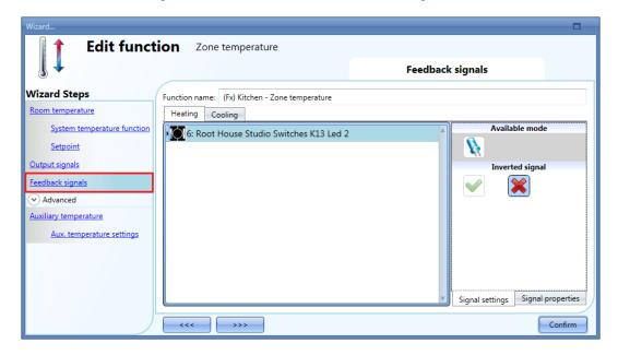
The inverted logic for the feedback can be selected in the Signal settings tab window.
