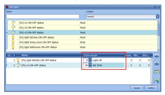
The user can also change the action of the function in the sequence functions window.
