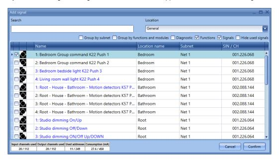
Select the signal/signals you want to use as *Group command*. If more than one signal is selected in this window (you can choose up to 20 signals), the function will be activated/deactivated if at least one signal is active (the system performs the logical OR).
