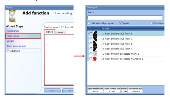
Each time the reset signal is activated, the counting value is reset.
