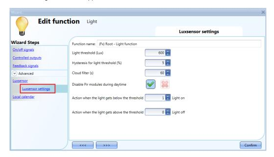
In the field *Light threshold (lux)*, the desired daylight level below which you want your light ON must be entered. A value between 0 and 5000 lux can be set.
