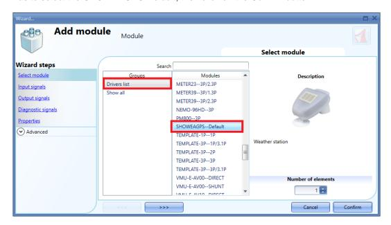
To configure the serial parameters of the weather station, click on the relevant picture once it is added to the project:
