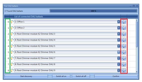
*New discovery* assigns a new address to each ballast, as shown in the first column (see the green rectangle). Each ballast can be switched on/off by means of the toggle button shown in the red rectangle. The installer can use this function to locate the ballast and give it its proper name.
