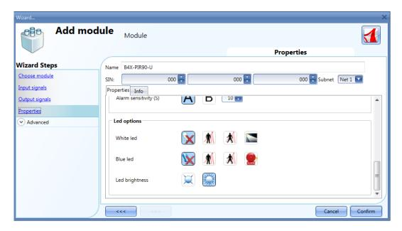
In this window the sensitivity has to be configured, also the behaviour of the LEDs: they could be used as a guide light, feedback on the detection of presence or movement or feedback of an alarm.
