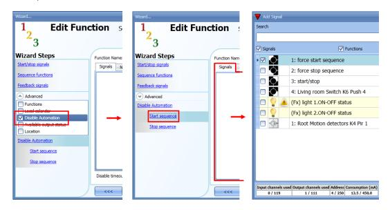
Each signal used in the *Start sequence* window works in level mode. Until the start signal is active, the function is executed and cannot be deactivated until the start signal disappears.
