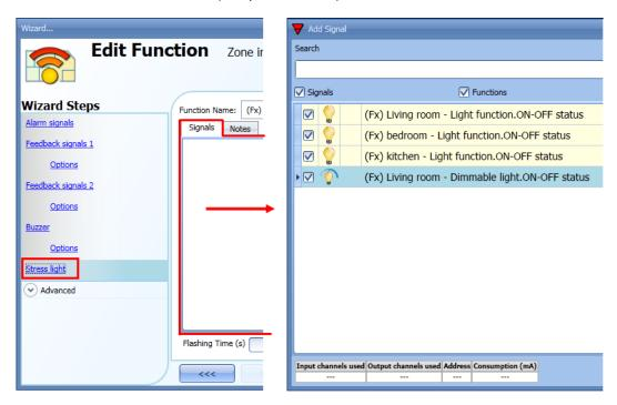
The *Flashing time* of all the lights added to the list has to be set at the bottom of the stress lights window (see picture below).
