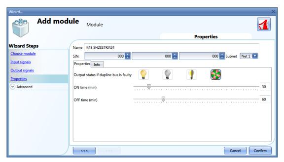
As for the setting of the output modules SH2SSTRI424 and SH2RE16A2E230, the user has to select the fail-safe working mode when the bus is faulty or not connected.
