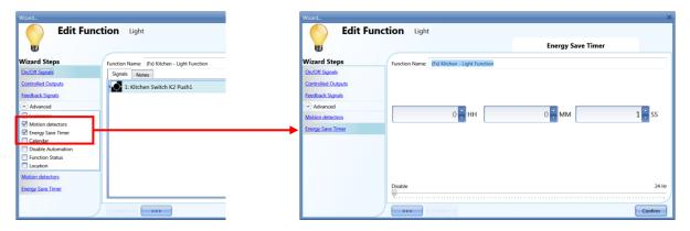
A minimum time of 1 second has to be set to switch the light OFF. You can set the desired delay off timer by moving the slider or by typing the hours, minutes and seconds.
