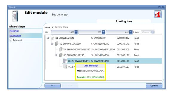
3. With the left mouse button held down, drag the object to the desired location (over the K4 SHJWD200WEWLS230 module as shown in the example below).
