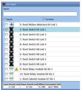
Once the alarm signal is entered, the user can also decide to use the inverted logic of the signal (see the red rectangle in the picture below). The inverted logic is enabled by selecting the green V.
