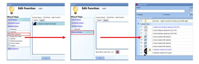
The *Motion detector* menu will appear. After selecting it, with a double click on the Signal window, the list of available signals will appear.
