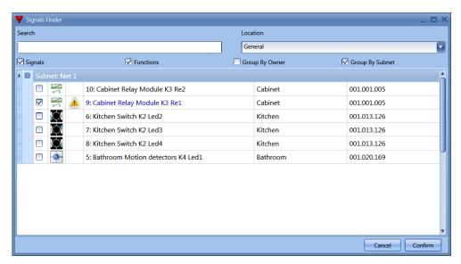
The signals available in this window are relays and LEDs. Up to 50 signals can be chosen and they are managed in parallel.
