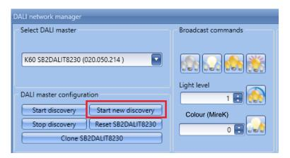
When the DALI network discovery starts, the master assigns a 24-bit random address to each ballast. This type of address can have values starting from 0 up to 16.777.214 ( $2^{24}$ -2).
