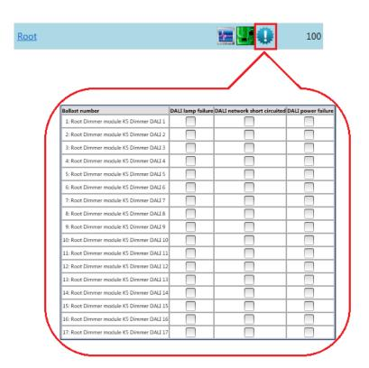
If a failure is present on the DALI bus, it will be shown by the icon turning orange and when the mouse hovers over the icon, a tool tip appears, flagging the relevant error. There is one line for each ballast.
