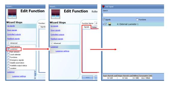
The user can add up to 10 lux sensors: if more lux signals are linked to the function, the average value is calculated and used.
