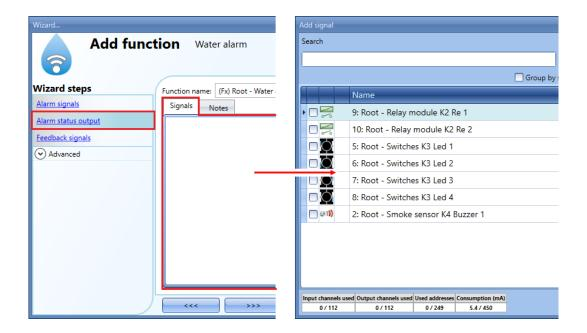
The output signal can be a relay, a LED or a buzzer. The output signal will stay on until water is detected by the sensor.
