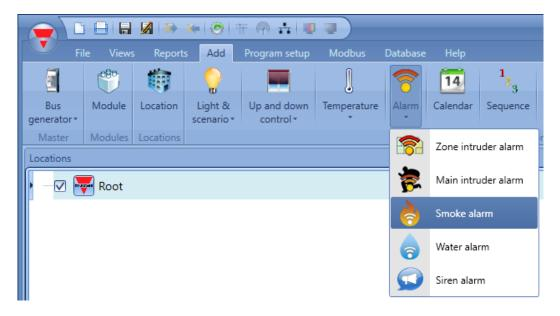
This function manages one or more outputs controlled by one or more input commands. The command might be a signal from a smoke detector, a pushbutton, a switch, a function or a remote command (Webserver, sms. Modbus TCP/IP)
