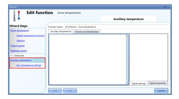
In the *Aux. temperature settings* of the function, the user can set two different thresholds: the *High temperature threshold* (over value) and the *Low temperature threshold* (under value). The *Hysteresis* and the *Delay on* time are applied to both the thresholds.
