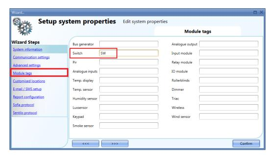
When a new light switch module is added, the name tag will be linked to a number that is increased each time a module of that group is added: for example, the first light switch module will be preceded by *SW1*, the second one by *SW2* and so on so forth (see picture below).
