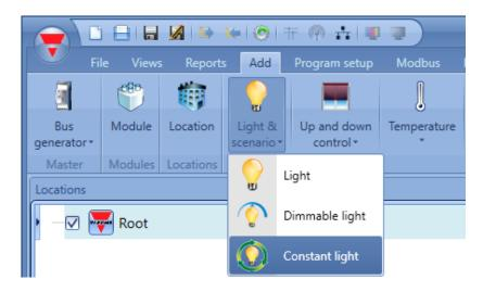
This function manages one or more dimmer outputs controlled by one or more input commands. The command might be a real signal such as a pushbutton, a function or a remote command (Webserver, sms, email, Modbus TCP/IP)
