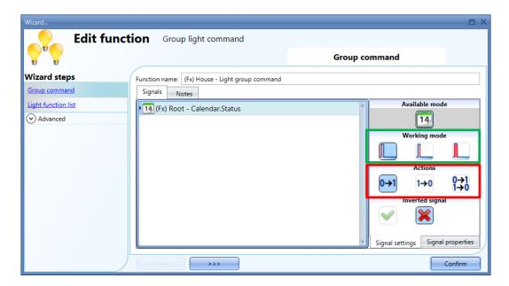
The signals of this type perform the selected action when they change level, according to the table below:
