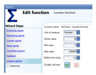
In this window, the user has to set the *Reset value* of the counter at start-up, the *maximum* and the *minimum* values the counter is to have and above or below which the counter will not go, and the *Delta time*, which is the interval time used to calculate how much the counter has been increased.
