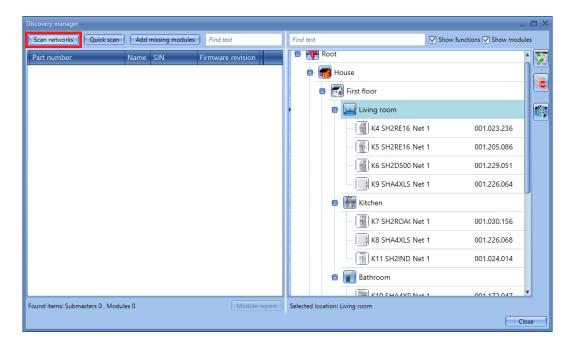
Once the scan is finished, the UWP 3.0 tool will present the list of devices found, grouped according to the Dupline network they are connected to. This means that the system also shows which Dupline generator SH2MCG24 each module is connected to.
