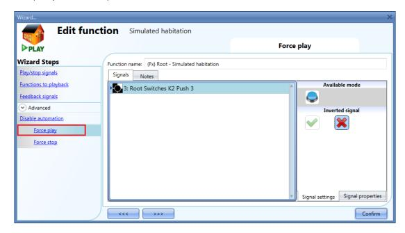
Each signal used in the *Force play* window works as a level signal. Until the signal is active, the function is forced to play.
