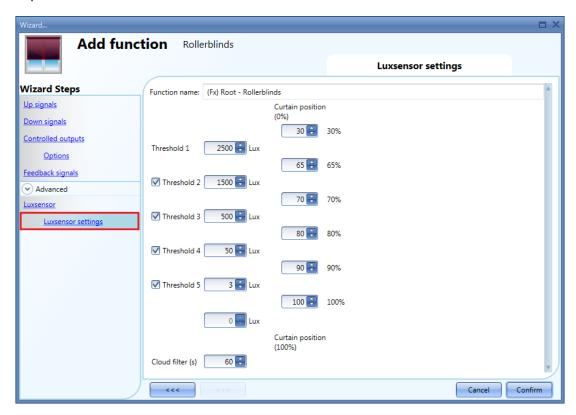
The up/down movements and the tilting start when the thresholds are surpassed, so if the blind position is changed manually by means of a light switch or automatically e.g. by the scheduler, the automation of
