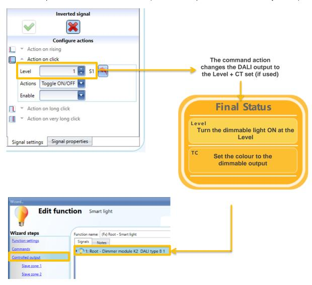
To select the output signal that is controlled by the Smart light function, click on *Controlled output* and then double click on the Signal window. Once the output window is opened, select the relevant outputs from the list.
