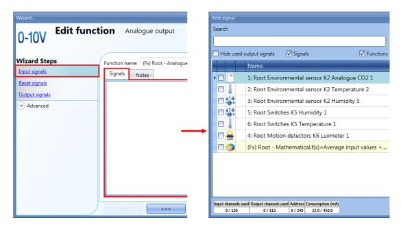
Only one input signal can be added to the Analogue output function
