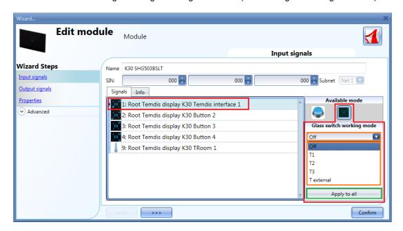
The Glass switch working mode can be configured as shown in the following steps.
