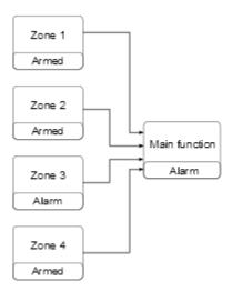
If the alarm input signal is no longer active, the previous alarm condition is still saved and the status of the main function is "Waiting for acknowledgment" to advise the home owner that an intrusion has been detected. This status is reset when the main alarm function is disarmed.
