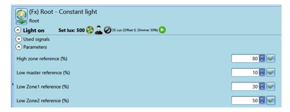
In the example shown above, when the master zone output is set to 10%, slave zone 1 will be set at 30%, while zone 2 will be at 50%.
