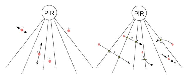
The pulses generated by the PIR (i.e. the detection of a change in temperature) are compared with a threshold temperature value.
