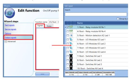
The output signal can be a relay or a remote control switch, and it follows the status of the function: when the function is ON, the output will be activated, when the function is OFF, the output will be deactivated.
