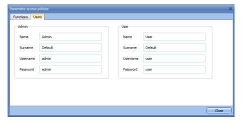
The username and password for the *Admin* account can only be changed by using the Tool, while those for the *User* account can be changed by means of the UWP 3.0 tool and the webserver.
