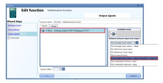
The 0-10 V output value is calculated based on a linear relation between the minimum and maximum values of the function: in the Signal properties window of the output, the user can set the Virtual range (0 - 100) and the Output range (0-10 V) according to the project, as explained in the picture below:
