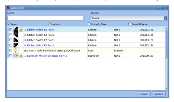
Select the signal/signals you want to control your light with. If more than one signal is selected in this window (you can chose up to 50 signals), the function will be activated/deactivated if at least one signal is active (the smart-house system does the logical OR).
