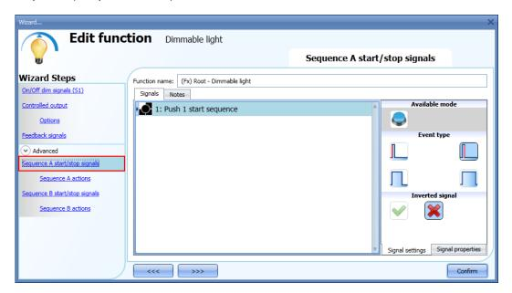
The sequence is stopped when any dimmer command is generated. For each signal the inverted logic can be enabled.
