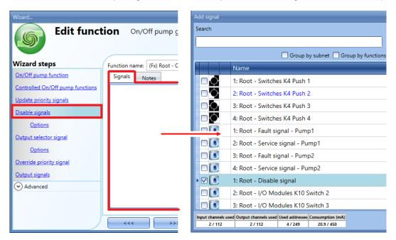
If a level signal is selected, such as a switch, or a function, the available actions are **Action on rising** (i.e. when the switch is closed or the function is activated), **Action on falling** (i.e. when the switch is open or the function is deactivated), or both. The inverted logic for the **Disable signal** can be enabled by selecting the green V in **Inverted signal** (see the green box below).
