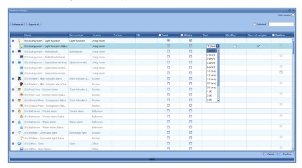
The *Database manager* window allows the user to add the signals, such as analogue and digital signals and function statuses, to the Database of the UWP 3.0. For each signal there are different options to store its value to the Database, as described below:
