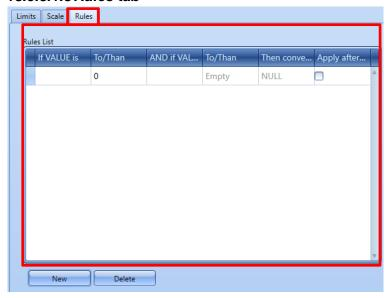
In the *Rules* tab, the user can enter some instructions to filter or manage the read values. This operation can be done before and/or after having scaled the raw values.
