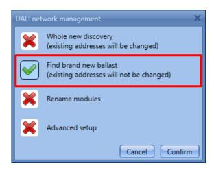
This function performs a new network scan, leaving unchanged the ballasts already configured.
