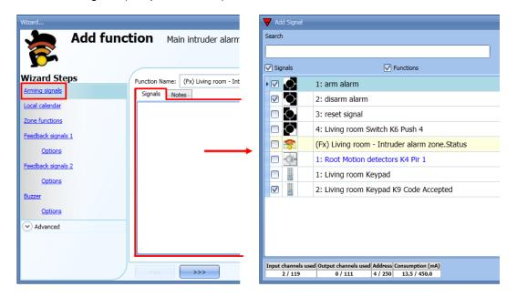
When the arming signal is activated, all the linked zone functions are automatically armed; each zone is armed according to the arming time set by the user.
