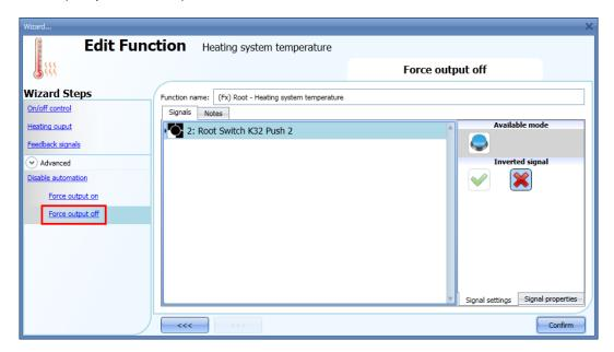
Each signal used in the Force output off window works in level mode: until the signal is active, the output stays off.
