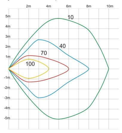
Figure 5: Vertical sensitivity area.
