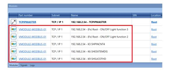
All the imported modules/functions are treated in the same way as the modules/functions connected to the master device and can be used in any logic.
