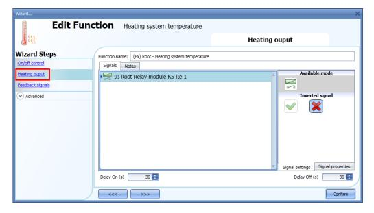
Once the output signal is added, the user can set two delays (delay on/off) to control the activation/deactivation of the system output (pump) and the zone output (valve) when a request for heating/cooling is received from a zone.
