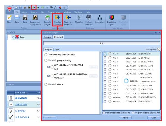
In this case, the system selects the objects to be programmed and the user cannot change anything. Only the memory of new modules will be programmed, while as for the other already existing modules, only the address will be programmed.
