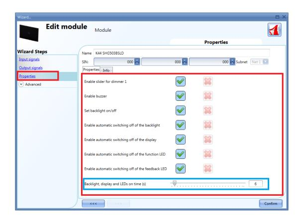
In the *Properties* field, the acoustic feedback and the backlight can be set as described here. The module has a built-in buzzer that can be enabled or disabled by the user: if it is enabled, when a key is pressed or the finger is moved over the slider, an acoustic feedback will be emitted. The glass has a backlight, two 7-digit displays, four function LEDs (L1, L2, L3, L4) and four feedback LEDs (FL1, FL2, FL3, FL4) which can be configured in this field:
