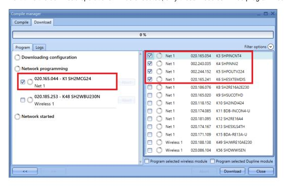
By clicking on the *Download* button, the system starts sending the project into the UWP 3.0. During this operation, moving or minimizing the *Download* window, it is possible to go on making changes to the configuration.
