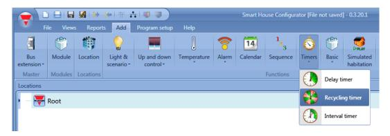
In the recycling timer function, until the trigger input is on, the output goes on and off with fixed timing. As soon as the trigger signal is activated, the output starts going on/off according to the Ton and Toff times; when the stop signal is activated, the output goes off.
