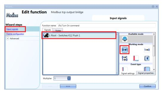
The Modbus TCP command will be sent when the push button is pressed, as shown in the red rectangle above.
