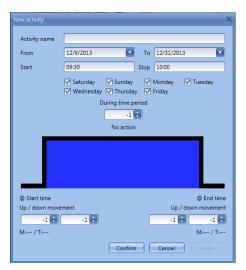
When the green V is selected, the activity menu of the calendar is changed, showing two actions at start time and at end time: the action for the up/down movement and the action for the tilting movement.
