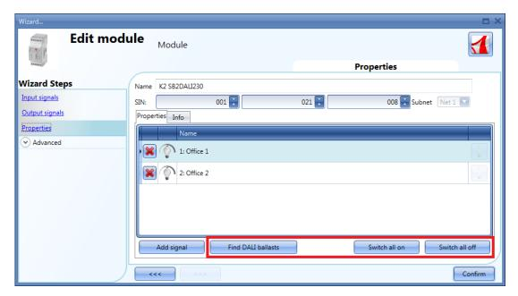
By means of the *Find DALI ballasts* button, the user can start a DALI network scan and the system will find the ballasts connected to the DALI bus.
