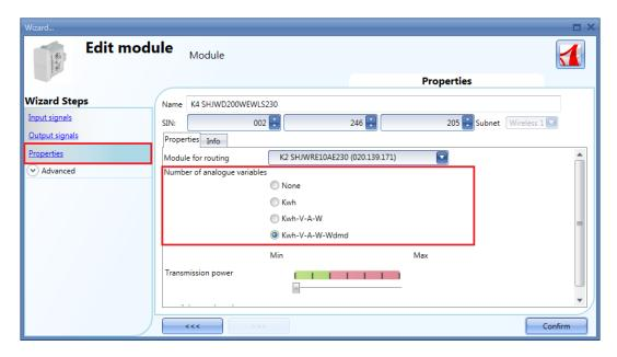
N.B. If the fourth option is selected in the field *Number of analogue variables*, the module will transmit the *kWh*, *V*, *A*, *W*, *Wdmd* values.
