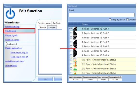
If more than one signal is selected in this window (up to 100 signals can be used) the function will be activated/deactivated if at least one signal is active (the system does the logical OR).
