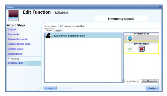
In the example below, the motor is stopped immediately when the emergency signal is activated.
