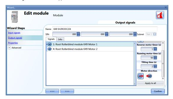
As for the setting of the roller blind module SH2RODC224 and the SH2ROCC224, the user has to set the Reverse motor time (the pause the motor takes before changing its direction), the Running motor time (the time the blind takes to go to a fully closed position from a fully open one) and the Tilting time (the time the motor needs to do a 180° rotation of the slats).
