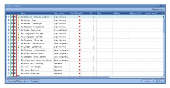
If the user clicks on the *expand/collapse* button, a selective selection of the signals (for modules and functions) can be done.
