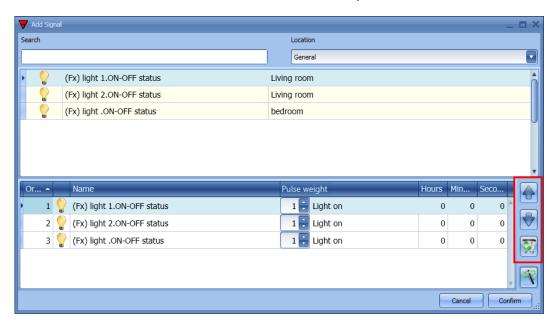
Using the icons on the right side of the window, the user can move up/down or delete a function from the list.
