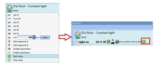
Once the set-up mode is enabled, the green circle with the "play" symbol will appear in the live signal window (red rectangle).
