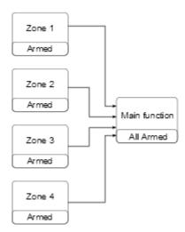
When all zones are armed, if an intrusion is detected in zone 3, the status changes to "pre-alarm" and then when the disarming time expires the zone goes into "alarm". The alarm status is transmitted to the main function and the main status becomes "alarm".
