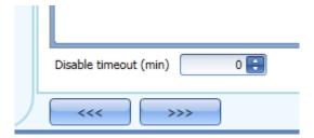
If the disable timeout is set to 0, the timer is disabled and the disable condition stays activated until it is removed manually.
