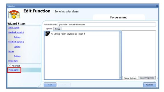
Each signal used in the *Force alarm* window works as a level signal. While the signal is active, the main alarm function, and all the linked zones, are forced into the alarm condition.
