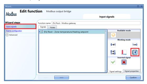
In the *Working mode* field of the Signals setting window, the *Every change* mode is selected (see the red rectangle above): whenever the *Zone temperature.Heating setpoint* signal changes, the Modbus RTU command will be sent to the Modbus device.
