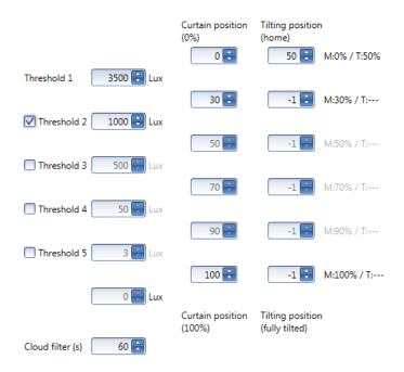
In the picture below, the behaviour of the output is shown according to the light level.
