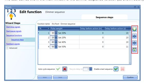
Using the icons on the right side of the window, the user can add, move up/down or delete a step from the list.
