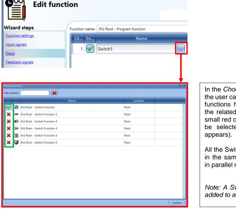
In the *Choose functions* window the user can select which *Switch* functions have to be added to the related step by clicking the small red cross, the function will be selected (a small *V* icon appears).
