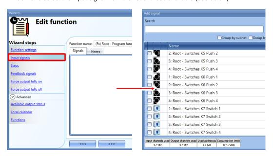
The available signals can be push buttons, switches and functions. The following table shows the actions available for push buttons:
