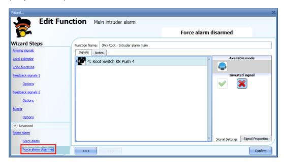
The alarm can be forced into disarmed in only a single zone by adding the *Force alarm disarmed* signal in the zone function (see picture below). An example could be a room of the house where the intruder alarm has to be disarmed even if all the other zones are armed (e.g. the room has some pets that could trigger the alarm).
