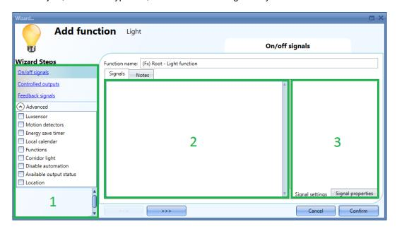
The wizard is a tool that drives the user in the configuration of an object, guiding them in small steps to the complete setup of a module, location or function. The aim of the wizard is to reduce the effort of understanding the complete process of a configuration, making it easy and fast. The different steps can be filled in one by one just by clicking on the ">>>" button and going through all of them, or by clicking on those required visualized in blue in the area on the right (Area 1).
