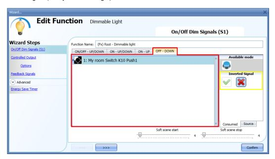
The user can set the soft scene start/stop: this is a common setting used for all input signals.
