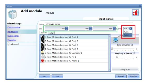
If a module is entered with a wrong Subnet, e.g. *Net1* instead of *Net2*, the user can click on the relevant picture from the Modules window, then the Subnet can be changed from the *Subnet* field of the *Edit module* window, as displayed in the red rectangle below.
