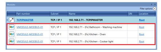
All the imported modules/functions are treated in the same way as the modules/functions connected to the master device and can be used in any logic.
