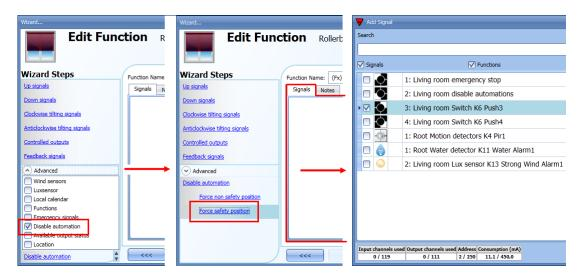
Each signal used in the *Force safety position* window works as a level signal: until the signal is active, the blind is forced into the safety position.
