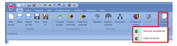
The user defines the modules and signals in a Template file. Customized names for modules and signals can be specified in order to override the default names provided by the UWP 3.0 Tool. The modules and signals list will be imported by an excel file provided by the UWP 3.0 Tool: when a new version of the software is released, the UWP 3.0 Tool embeds a new version of the file to manage new modules.
