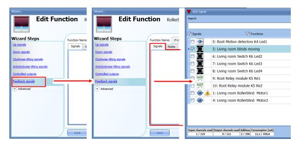
The signals available in this window are LEDs and relays.
