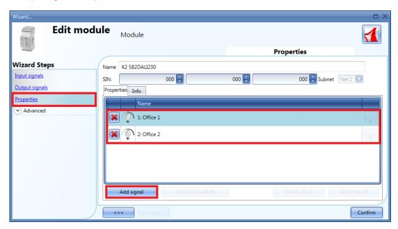
In the Properties window the user can add up to 64 DALI outputs for each SB2DALI230.
