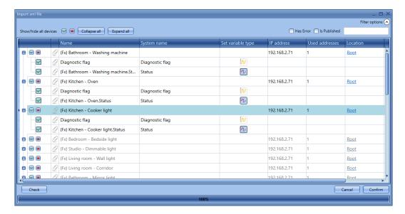
In the first column the user can select which functions and/or modules have to be added from the map of the Slave device: if the user clicks on the *small green V* icon, the selected modules/functions will be imported into the project; otherwise, if the user clicks on the small *X* cross, the selected modules/functions will not be imported. By clicking on the *Filter options* button, a selection of the variables is available.
