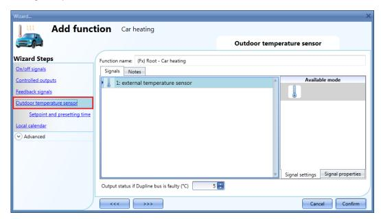
Should the temperature sensor be faulty, the system will use a default value that the user can set from - 50°C to +50°C.
