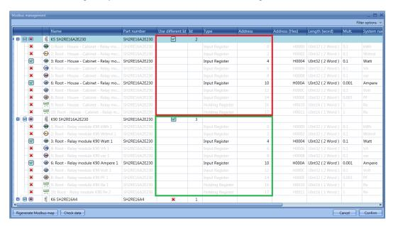
With the settings shown in the window above, the values read from the module SH2RE16A2E230 are always at the same addresses, and the user just needs to change the Modbus ID when he wants to read, for example, the power of the two modules.
