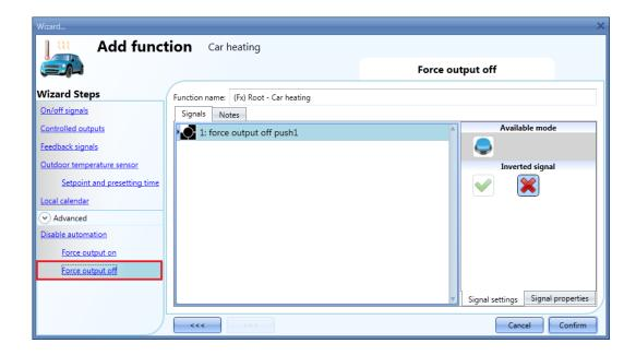
Each signal used in the *Force output off* window works as a level signal: until the signal is active, the car heating function is forced off.
