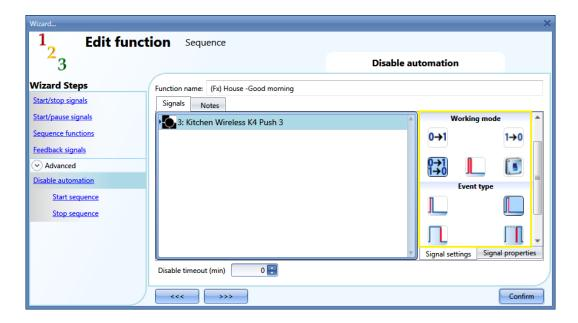
If a push button type is added, the working mode, highlighted by the yellow rectangle, has to be selected according to the table below:
