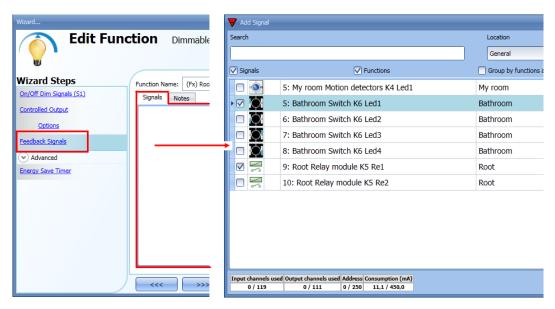
The signals available in this window are LEDs and relays.
