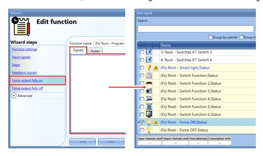
Each signal used in the *Force output fully on* window works in level mode. The behaviour when the signal is activated is as follows:
