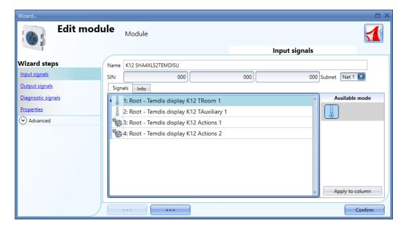
In the *Input signals* field, the temperature sensors, such as the *Troom1* signal and the optional *TAuxiliary1* signal, can be used in any temperature function.
