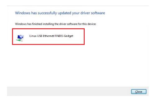
8. When the driver is installed, in the *Network adapter* category a virtual network board named *Linux USB Ethernet/RNDIS Gadget* will be added, as shown in the picture below. The driver automatically gives a dynamic IP address to the Controller/PC according to the actual IP of the PC.
