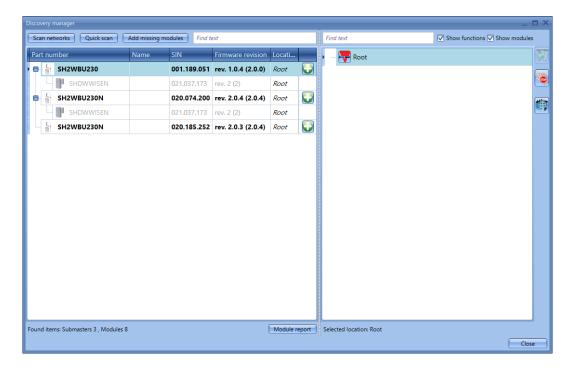
If more wireless base units are installed, the UWP 3.0 tool will show all the modules found in each network. If two or more SH2WBU230Ns cover the same area, they might find the same modules: it will then be up to the installer to associate the "orphan" modules to the required SH2WBU230N.
