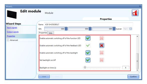
In the *Properties* field, the acoustic feedback and the backlight can be set as described here. The module has a built-in buzzer that can be enabled or disabled by the user: if it is enabled, when a key is pressed or the finger is moved over the slider, an acoustic feedback will be emitted. The glass has a backlight, two 7-digit displays, four function LEDs (L1, L2, L3, L4) and four feedback LEDs (FL1, FL2, FL3, FL4) which can be configured in this field:
