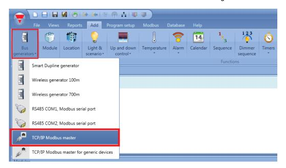
In the TCP/IP Modbus master interface the user has to define the IP address of the Modbus device which is to receive the commands sent by the UWP 3.0 controller.
