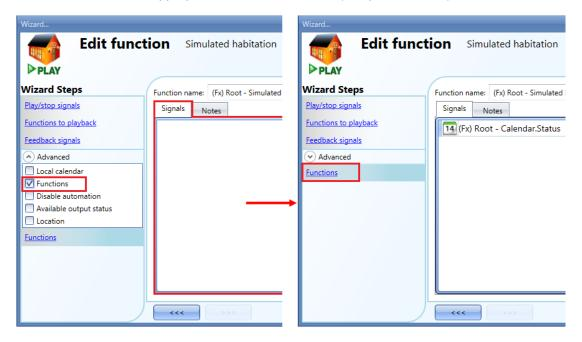
The playback of the simulated habitation acts according to the function status: when the function is active, the simulation is played; when the function is not active, the simulation is stopped.
