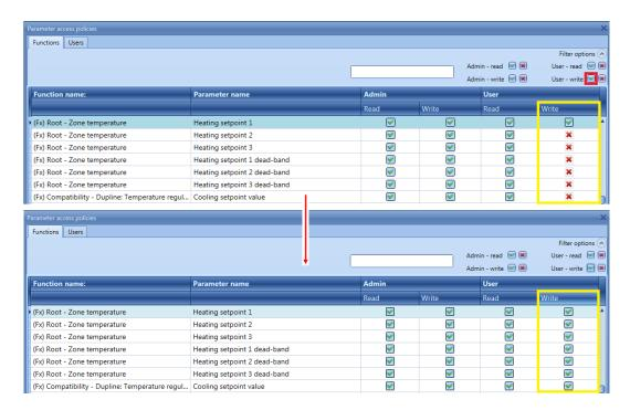
The access data for the two accounts can be configured by entering the *Users* window. The admin account (Admin) has a higher priority for the management of all the functions added: it has full access to all functions (all permissions ticked).
