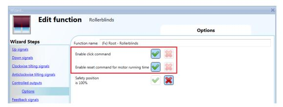
The reset command is also available via the webserver (when accessed as administrator) and via the UWP 3.0 Tool in the live signals mode. When the command is sent by using the webserver or the Tool, a window with a warning message is shown to advise the user not to stop it.
