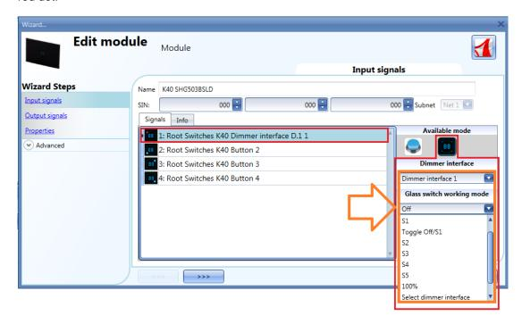
Since this panel can control up to 4 dimming functions, also called dimmer interface, each key can be freely associated to one of them. More than one key can be associated to the same dimmer interface (or dimmer function).
