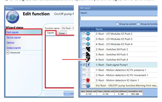
Once a fault signal is entered, the user can also decide to use the inverted logic of the signal. By selecting the green *V*, the inverted logic is enabled.
