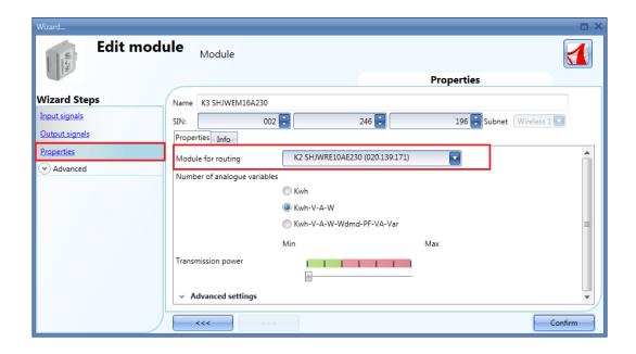
In the *Number of analogue variables* field, the user can select the relevant group of analogue variables, as shown in the red rectangle in the picture below.
