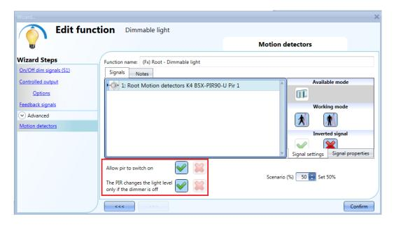
By using the above settings, the Dimmer function will work in this way: if the light is OFF and the PIR detects the movement, the light level is set to 50%, then it is possible to adjust the light level of the function using the pushbuttons, for example to 80%. When the light is ON and the light level is changed, the PIR doesn't set the 50% when the movement detected.
