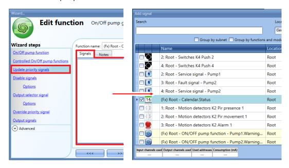
If a level signal is selected, such as a switch or a function such as a *Calendar*, the available actions are **Action on rising** (i.e. when the switch is closed or the function is activated), **Action on falling** (i.e. when the switch is open or the function is deactivated), or both (see the green box below).
