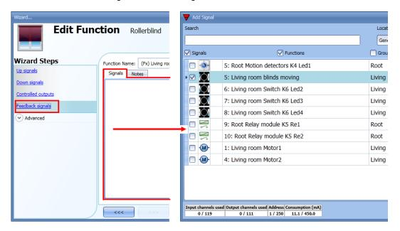
The signals available in this window are LEDs and relays.
