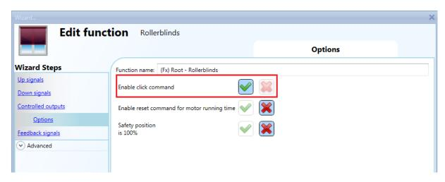
2) A long press (> 0,5 sec) activates the motor output until the input signal is ON (the blind goes up/down until the user keeps the pushbutton pressed or the selected signal is active). This functionality doesn't need to be enabled.
