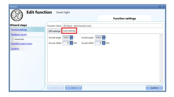
In the *Clock settings* tab, for sunrise and sunset times calculation, the user can set the angle of the sun below the horizon. The default value is 0.833 degrees for both *Sunrise angle* and *Sunset angle*. These values can be changed by the user considering the following indication:
