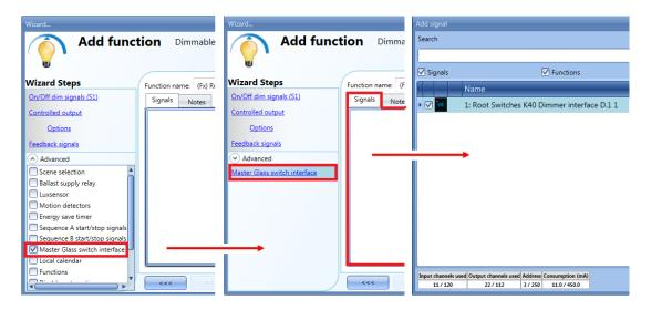
To use a key programmed as dimmer interface in a Dimmable light function, select *Master Glass switch interface* in the *Advanced* field, double click on *Signals* and select the required dimmer interface.
