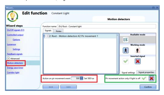
When the PIR does not detect any movement in the corridor, the light returns to the level set in the Corridor light options.
