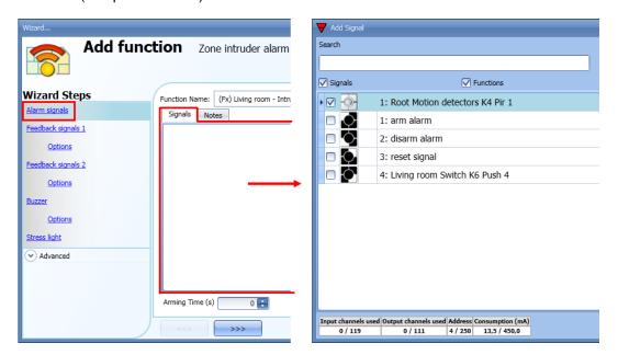
Once the alarm signal is entered, the user can also decide to use the inverted logic of the signal (see the red rectangle in the picture below). By selecting the green V, the inverted logic is enabled. Each alarm signal added to the function has a delay time that can be set in order to filter the activation of the alarm when a burglar is detected; this might be used to avoid false alarm triggering.
