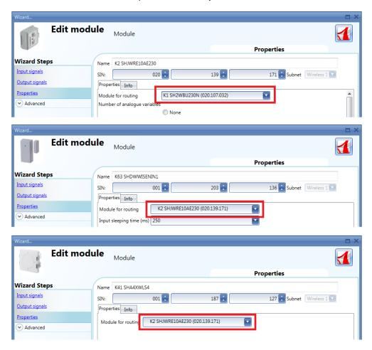
The picture below shows an example of an indirect connection where a wireless relay module is used as router.
