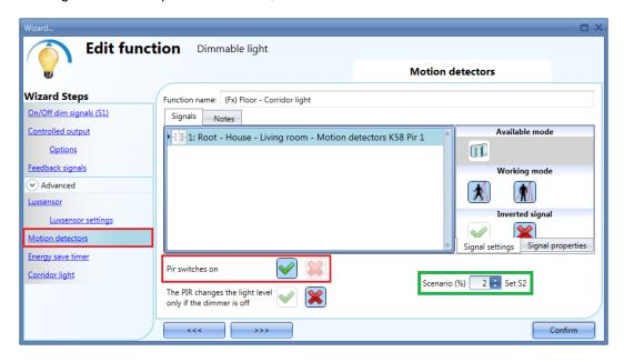
When the PIR does not detect any movement in the corridor, the light returns to the light level set in the
