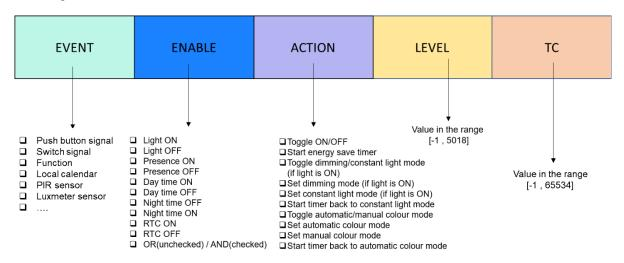
The Smart light function, whatever type of control has been chosen (Dimmable light, Constant light), is an **Event controlled** function: as soon as an **Event** occurs, such as a *Push button click* or an *RTC ON* signal, the DALI ballast output changes its status (the **Level intensity** + the **Colour temperature** value), according to the settings.
