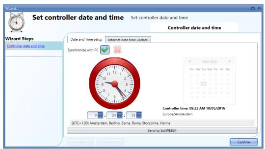
By clicking on the green V, *Synchronise with PC* and by clicking on *Send to UWP 3.0*, the Tool synchronizes the UWP 3.0's clock with your PC clock. If your PC clock is not correct, this time error will be transferred to the controller.
