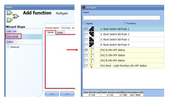
Once the input signals are entered, the user can also choose to use the inverted logic (see yellow rectangle in the picture below).
