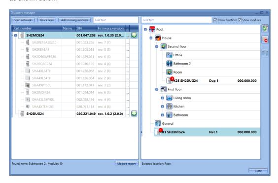
For each Master-generator, such as the SH2MCG24, SH2DUG24 or SH2WBU230N that have been found, the system shows a small red icon ( over a module where an association can be made.
