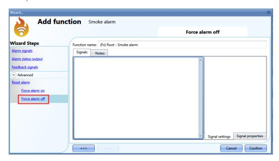
The signal used in the *Force alarm Off* window works as a level signal: while the signal is active, the function is forced to the Off condition (the output stays off).
