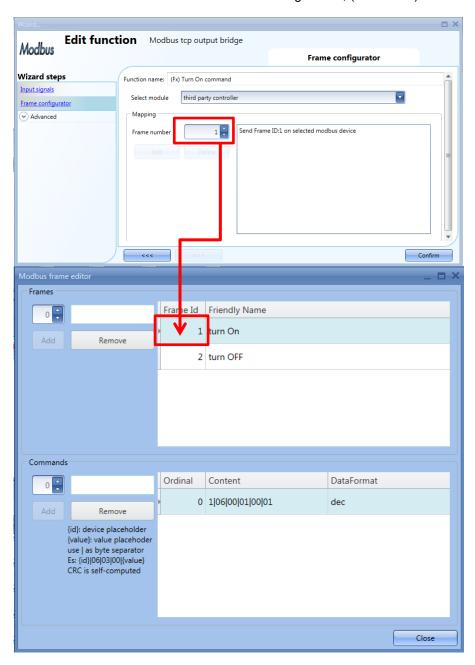
As a result of this configuration, each time the pushbutton is pressed, the Modbus TCP command *Turn ON device* will be sent to the Modbus device selected in the *Modbus TCP output bridge* function.
