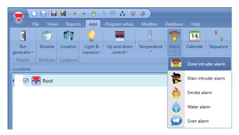
Once the zone alarm is added, the user has to select *Alarm* from the Add menu, then select *Main intruder alarm* (see picture below).
