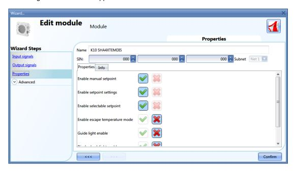
In the Input signals field, the available temperature values are shown, and the only window with the configuration settings is *Properties*.
