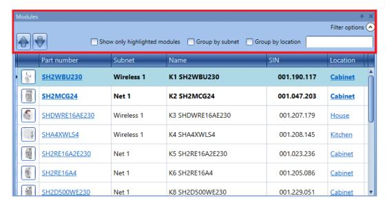
Only the modules specified by the filter will be presented: the filters can be used individually or they can be mixed.
