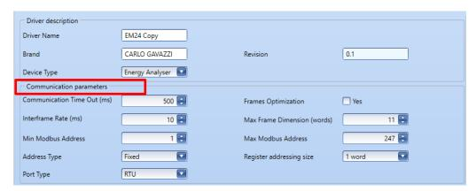
The user has to refer to the *Modbus map* of the device provided by the manufacturer to correctly set the different parameters.
