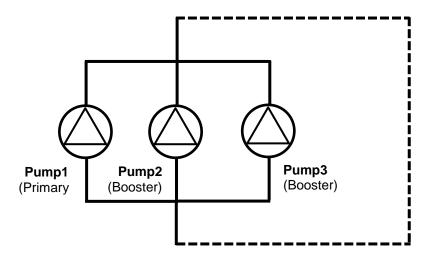
The number of outputs (the number of pumps that have to be activated in parallel) can be dynamically defined by an analogue input signal in the range of 0..10V, called the *Output selector signal*.
