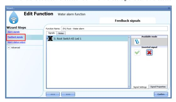
Once the alarm signal is entered, the user can also decide to use the inverted logic of the signal (see the red rectangle in the picture below). The inverted logic is enabled by selecting the green V.
