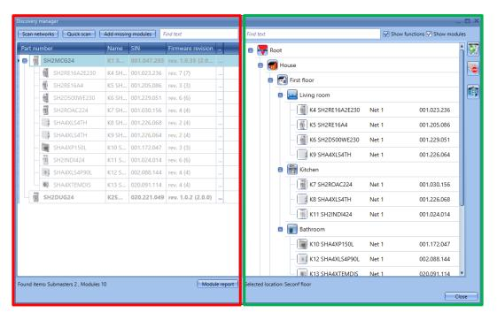
On the left of the window (marked in red), all the modules connected to the bus are prompted once the *Scan networks* push button is pressed.
