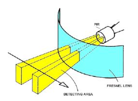
When a warm body moves into the sensor's field of vision, the sensor detects a difference in the measured temperature.
