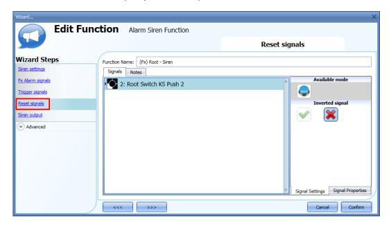
When the reset is activated, the siren is inhibited and stays in this condition until another alarm signal triggers the siren.
