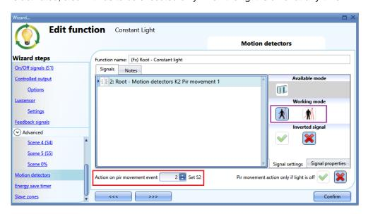
The action has to be selected in the field Action on PIR movement event according to table A:
