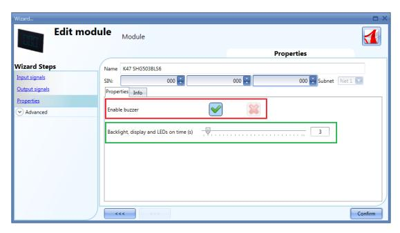
In the *Properties* field, the acoustic feedback and the back light can be set as described here.
