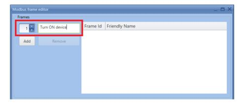
Each added frame has a specific identification number (*Frame id* field), which is used to identify the Modbus TCP command in the *Modbus TCP output bridge* function (as illustrated in the next paragraph).
