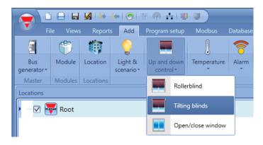
This function manages one or more motor outputs controlled by one or more input commands. The command might be a physical signal like a pushbutton, a switch, a function or a remote command (Webserver, sms, Modbus TCP/IP).
