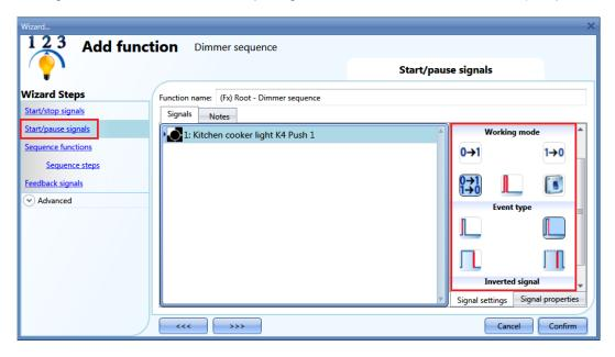
The input signal can be used either to start and/or to pause the sequence. When the sequence is paused, a start event will activate the sequence from the step where it was paused.
