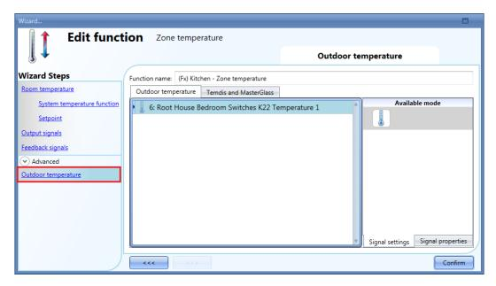
Two different types of signals can be used: in the *Outdoor temperature* signals window, the user can add one or more temperature signals from the sensor modules (e.g. BSI-TEMANA-U, SHA4XLS4TH, SHE5XLS4TH, SHGxxxW-BLSx). In the *Temdis and MasterGlass* signals window, the user can select to use the TEMDIS "T Auxiliary" signal.
