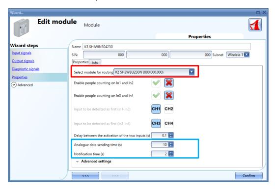
In order to limit the traffic of data between the wireless base unit and the Wireless input module, in the *Analogue data sending time* (s) field the user can set the period in seconds in which the analogue values are sent to the UWP 3.0 Tool.
