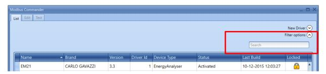
The user can enter the search criteria and the system will provide all the searched *Modbus drivers*: these can be sorted in ascending or descending order by clicking on the header fields.
