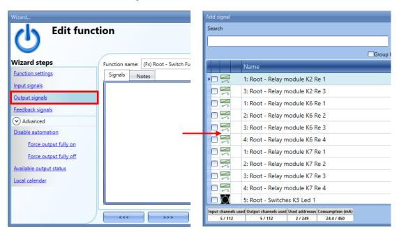
The signals available in this window are relays and LEDs.
