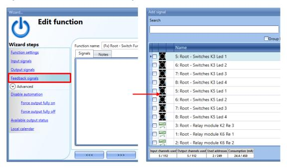
The signals available in this window are LEDs and relays. Up to 50 signals can be chosen and they are managed in parallel.
