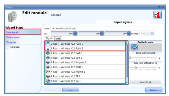
The SHJWRE10AExLS230 module integrates two programmable capacitive push-buttons and can be used in all the UWP 3.0 tool functions, as shown in the red rectangle in the picture above.
