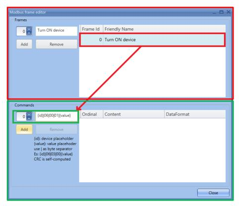
In the *name* field of the *Frames* area, the user has to enter the name of the Modbus RTU command, as shown below:
