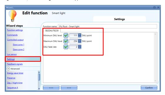
By clicking the green *V* icon, the user can set in the *DALI fade rate* field a specific value, as shown in the example below:
