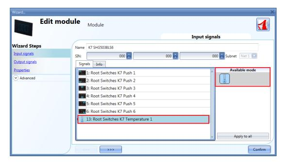
The SHG503WLS6 and SHG503BLS6 are glass switches with temperature sensors that can be used in any temperature function.
