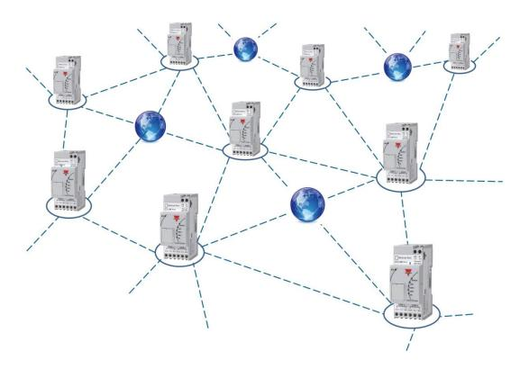
Each UWP 3.0 can be a Modbus master and a Modbus slave device at the same time. An UWP 3.0 can read and write values from/to other Sx2WEB/UWP 3.0s, but can only read from VMUCs.
