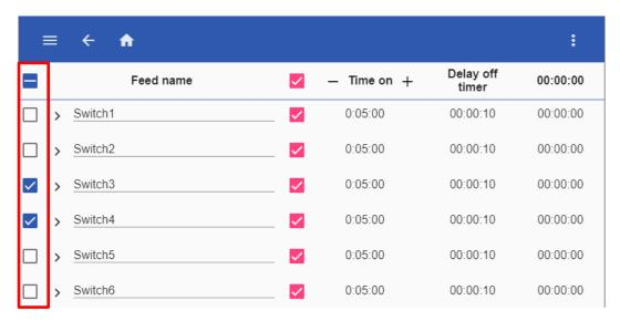
Note: To enable/disable all the steps at the same time, the user can click on the  $\checkmark$  in the column header.
