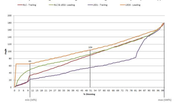
In this example the lighting circuit turns on at a phase angle of 66° (if 60° is the minimum angle to switch the lamp on, 66=60+10% is the minimum angle to switch it on without any flickering). Afterwards, if the minimum dimmer output is set at 50%, the minimum switching on angle will be 104° (see the graph above).
