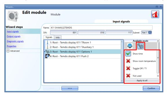
By means of the Available mode list, the user can associate the key to the required function:
