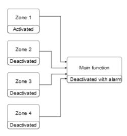
The home owner leaves the house and uses the keypad placed in zone 1 to arm the alarm.
