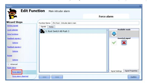
The alarm can be forced in only a single zone by adding the force alarm signal in that specific zone function (see below).
