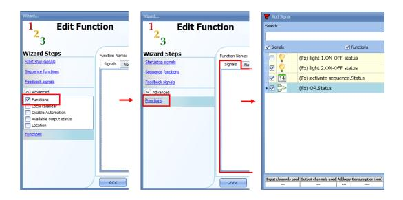
All the added functions will trigger the sequence according to the status they have: for example, a light that is switched on will make the sequence start; the same function that is switched off will make the sequence stop.
