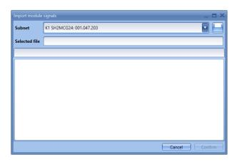
In the **Subnet** list in the window, the user has to select which Subnet the modules have to be attached to: **only the SH2MCG24** Master Channel Generator is allowed. One file permits specification of the modules attached to only one network. To manage multiple Subnets, one Template file has to be created for each Subnet of the project.
