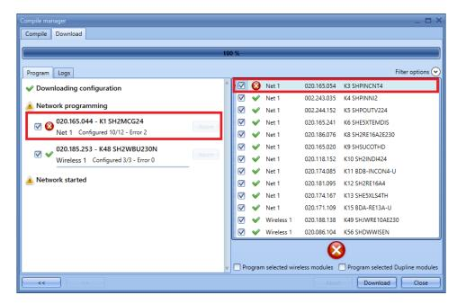
The selective download functionality detects automatically what are the modules that have not been programmed, so they will be selected automatically next time the *Compile project* function is executed. As displayed in the picture below, the faulty module *K*3 is ready to be re-programmed.
