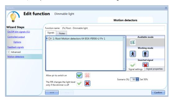
Every time the PIR detects movement, the light level is set to 50%, regardless the previous level reached by the function.
