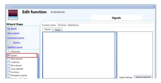
To add the signal to control the Up/Down movement, the user should click on the relevant section, then double click on the *Signals* window and select the input signal from the list.
