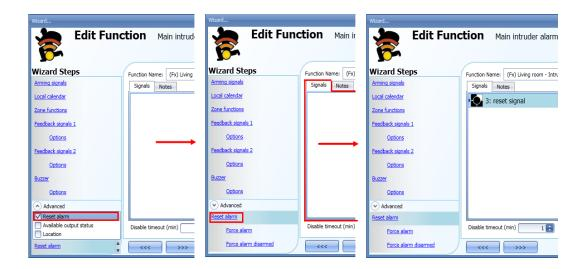
The reset signal can be managed as an event signal or a level signal: the event signal triggers the *Disable timeout*. When the alarm is reset, at the end of the Disable timeout, all the zones will be armed again.
