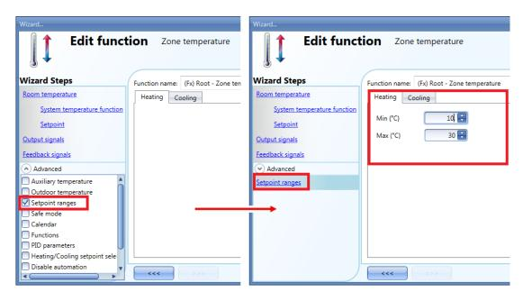
To change the predefined set point values, the user should click on the relevant field in the wizard of the zone temperature function. In the Advanced section, in *Set point ranges*, the user can select the operating range for the set points (min is 10°C and max is 30°C by default).
