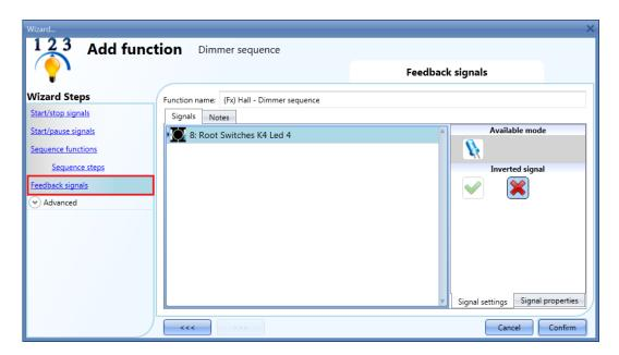
Once the feedback signal is entered, the user can also select the inverted logic.
