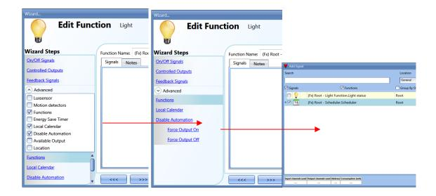
If the calendar is programmed as "a calendar for level signal", it has to be added in the On/Off signal field.
