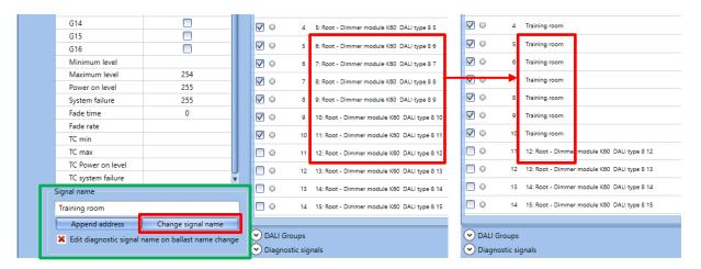
By clicking on the *Append address* button, the *short address value* will also be added to the new signal name:
