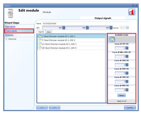
In the *Output signals* field the user can set the output curve according to the input voltage level required by the connected load. The curve is divided into six steps (OFF, 10%, 30%, 50%, 70%, 90%) and for each step the voltage level can be defined.
