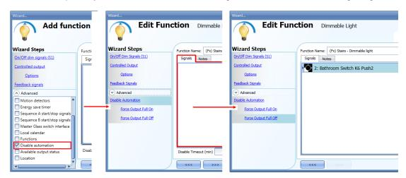
Each signal used in the Force output fully off window works in level mode.
