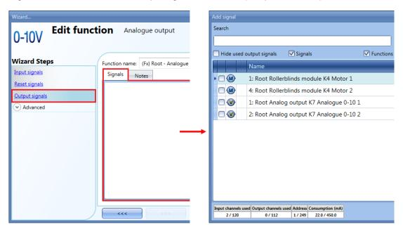
The running parameters of the rollerblind modules can be set directly from this wizard, in the *Signal properties* tab window, without the need to re-open the wizard of the module.
