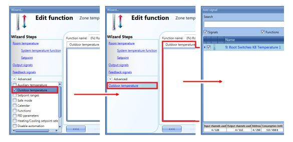
To add the external temperature signal, the user should select the relevant section in the wizard of the zone function, then double click on the Signals window and select the *input signal* from the list of those available (see picture below).
