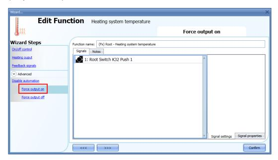
Each signal used in the *Force output on* window works in level mode: until the signal is active, the output stays on.
