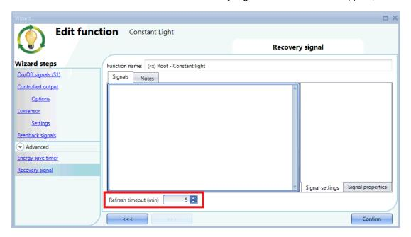
In the *Refresh timeout (min)* field the user can define a timeout value: when this timer expires the function automatically sends a command to the ballast and aligns the DALI outputs with the function status. This timer is restarted every time there is a manual action; when the timer expires, it is automatically restarted and cycles continuously. The value of this field can also be changed via the Live signals.
