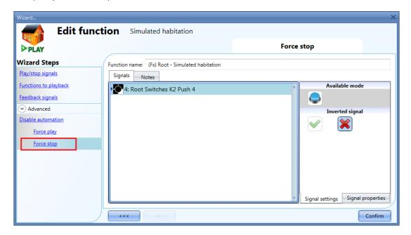
Each signal used in the *Force stop* window works as a level signal. Until the signal is active, the function is forced to stop (no simulation active).
