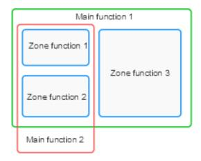
The "main alarm function 1" is used to arm/disarm all the zones (all zones must be linked in the function). For example, the alarm signal could be the keypad at the entrance of the house, used for arming the entire system when the user leaves the house.
