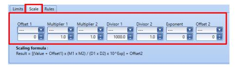
In the *Scale* tab, the user can enter some coefficients to process the raw read value according to a predefined equation, in order to get the actual value.
