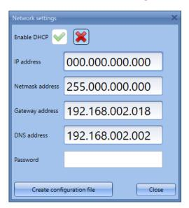
Once you have entered the required field, click on *Create Configuration File:* the UWP 3.0 Tool will create the file *controller\_settings.shcfg for UWP 3.0 Tool and controller\_settings.shcfg* for UWP 3.0 Tool that you must copy into a USB stick or a microSD.
