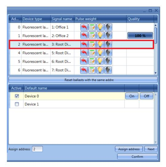
The user can then move to the next device to be addressed by clicking on *Next*. To save the new address click on *Confirm*.
