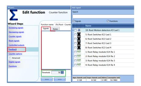
The selected signals will be on if the counter is greater than a configurable threshold, otherwise it will be off
