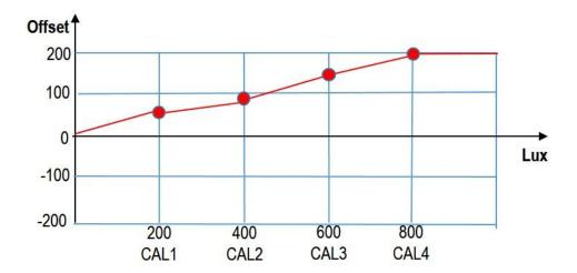
In the example shown above, the calibration has been carried out according to the four scenarios set at 200, 400, 600 and 800 lux, and for each of them the relevant offset of 50, 90, 140 and 200 have been calculated. From these four points a line is built and this is used by the constant light algorithm to calculate the correct setpoint at each light level. For this reason, it is important to calibrate the function at the light levels that will be used in the office.
