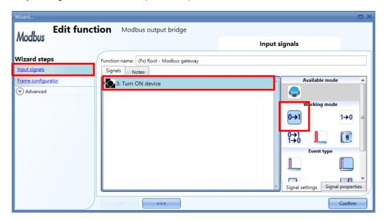
The Modbus RTU command will be sent when the push button is pressed, as shown in the red rectangle above.
