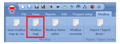
The *Modbus management* window allows the user to configure the signals to read and write via Modbus. They are split into two groups:
