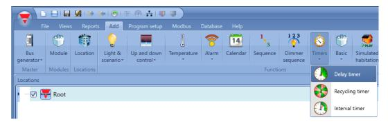
Using the delay timer, the output replicates the status of the input, applying a delay On and/or a delay Off time.
