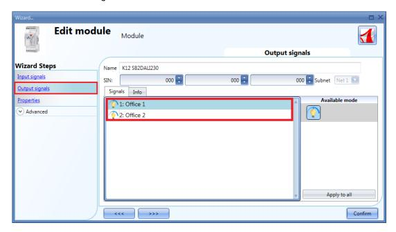
In the Output Signals window, all the DALI dimmers added in the Properties window will be shown.
