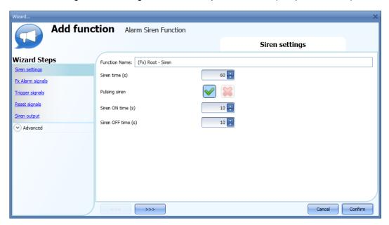
With the Siren time the user can define the activation time of the siren output when it is triggered by an
