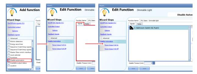
Each signal used in the "Force output fully on" window works in level mode. Until the signal is active, the light is forced to the fully on status. When the signal is non-active, the light returns to the previous status. When the *force to fully on* signal is activated and at the same time the *force fully off* signal is activated, the *force to on* status has priority.
