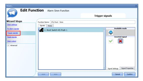
The behaviour of the signal used as the trigger works in the same way as described for the alarm functions: as soon as the trigger signal goes on, the siren is activated and stays on until the siren time has expired.
