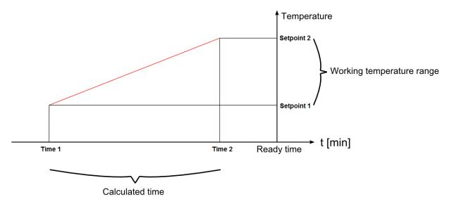
If the outdoor temperature is lower than or equal to *Setpoint1*, the heating is activated a *Time 1* before the *Ready time*. If the temperature is above *Setpoint2*, the heating is never activated. If the measured temperature is between *Setpoint1* and *Setpoint2*, the activation time of the heating output is calculated using the straight red line.
