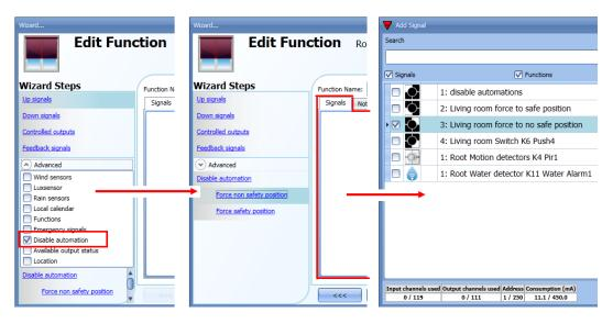
Each signal used in the *Force non-safety position* window works as a level signal. Until the signal is active, the blind is forced to the non-safety position.
