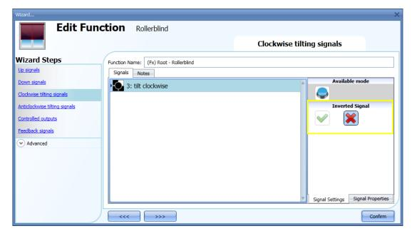
All the selected signals in the *Clockwise/Anticlockwise tilting signals* window work in parallel (they are managed in an OR logic).
