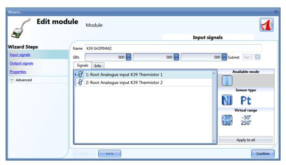
From this window the user can select the type of sensor connected to this input module and the input range.
