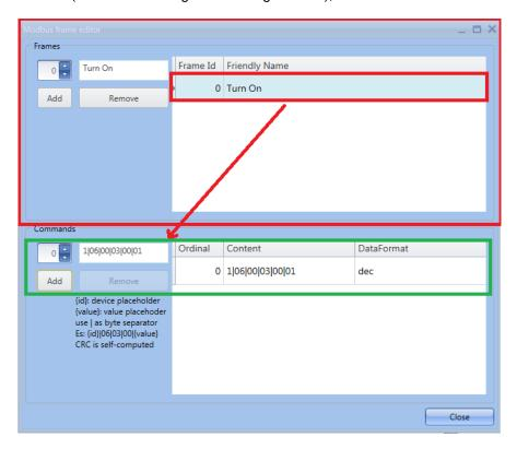
In the *name* field of the *Frames* area, the user has to enter the name of the Modbus TCP command, as shown below:
