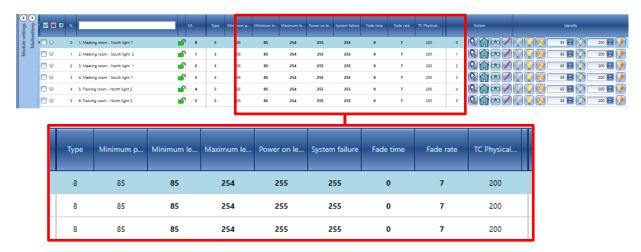
Every time a change is made, the dot next to the DALI ballast will be coloured in red: this means the data is not synchronized between the settings in the UWP 3.0 tool and the data in the DALI ballast. See the example below:
