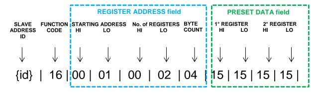
Following the two examples above, a Modbus command must be built using sets of characters separated by the "|" symbol (vertical bar). Each set of data has a specific position and must be edited according to the specifications below:
