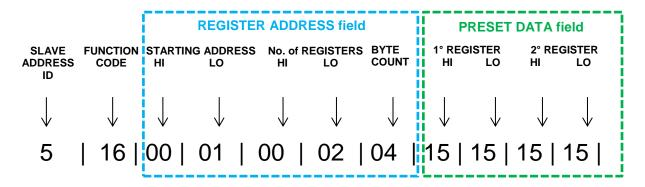
Following the two examples above, a Modbus command must be built using sets of characters separated by the "|" symbol (vertical bar). Each set of data has a specific position and must be edited according to the specifications below:
