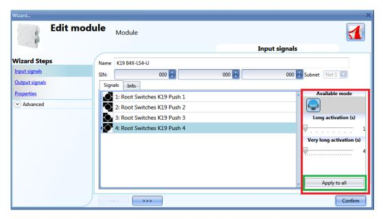
In the Input signals field, the Long activation and the Very long activation time has to be defined.
