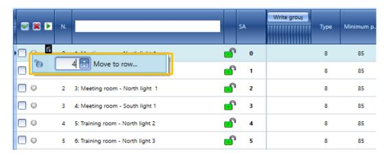
To swap two ballasts, enter the value of the destination row in the text box and press the *Move to row...* button. The selected row will be moved to the new row, as shown in the example below:
