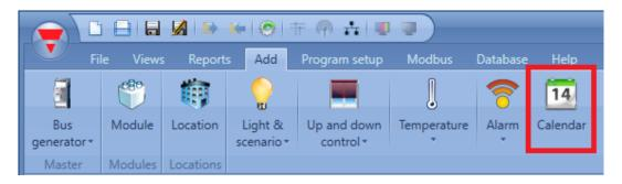
The calendar function can be used to perform different actions: for example, an external calendar could be created in order to switch off all the lights in an office at the end of the day, or move down all blinds at a certain hour in the evening.
