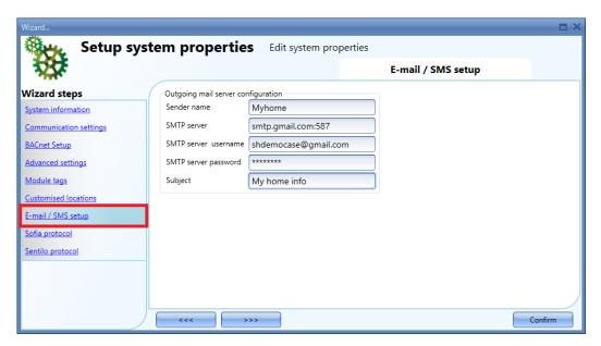
The user must enter the *Sender name* by typing the name used for the sender (e.g. My home). The user must complete *SMTP server* with the address of the server used for sending the email. The user must complete *SMTP server username* with the email address used for sending the email. The user must complete *SMTP server password* with the password for the email account. The user must complete *Subject* with the name used as the subject for outgoing emails.
