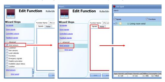
Once the wind sensor is added, the user has to set the wind speed limits in the Wind speed menu:
