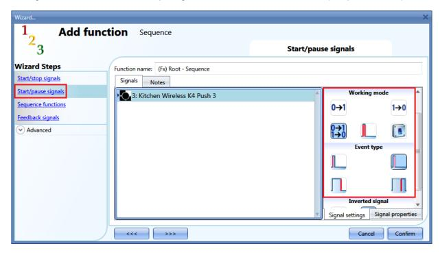
The input signal can be used either to start or to pause the sequence. Every time the sequence is started, it starts from where it was paused.
