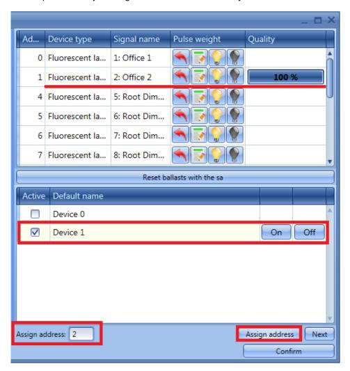
The ballast that was present in the window at the bottom (Device 1), is now present also in the window at the top with the newly assigned address as shown in the picture below (2 Fluorescent lamp).
