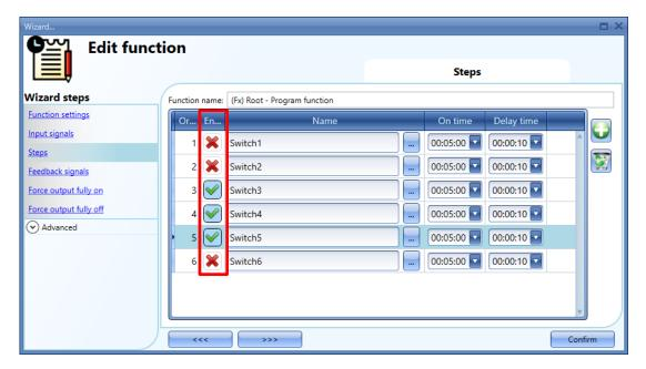
Click on the *Confirm* button, then in order to save the changes the next time the *Program* function is started, the user has to download the configuration to the UWP 3.0 controller by clicking the *Send to controller* button.
