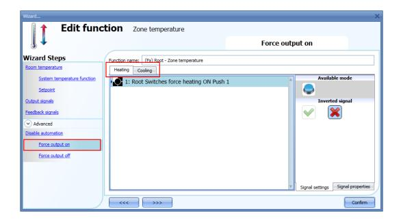
Each signal used in the *Force output on* window works as a level signal. Until the signal is active, the heating/cooling output is forced on.
