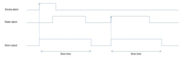
If the user needs to use different activations of the siren, in order to recognize the kind of the alarm triggering it, he must use different siren functions linked together with a multigate function.
