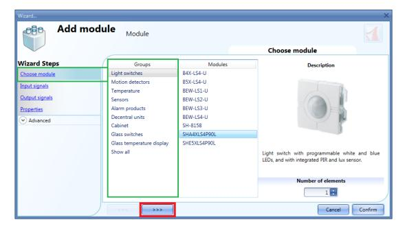
All the modules are added to the project with SIN 000.000.000, which can be set manually: this means that the installer can fill in the SIN by hand in the fields marked with a green rectangle. The SIN can be found on the module, on the box and on the label delivered with each device, it could also be attached to the manual or in the location where the module is placed.
