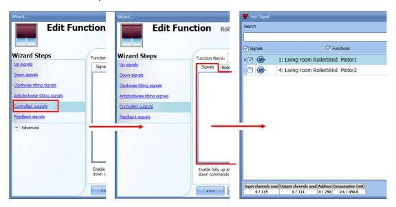
The signals available in this window are only the motor output type. Up to 10 motor outputs can be chosen and they will be managed in parallel.
