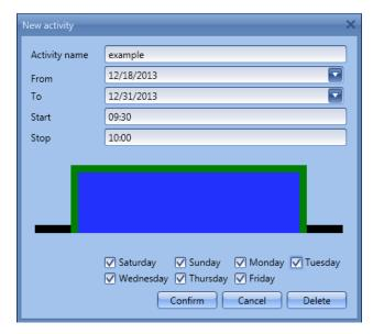
In the next picture a global calendar function is used to enable the input in a multigate function: the output signal is activated when the enable input is on and the pushbutton is activated. At 9:30 in the morning, the calendar signal goes On (multigate input 1 enabled) at 10:00 in the morning the calendar signal goes off (multigate input 1 disabled) and the output is switched off.
