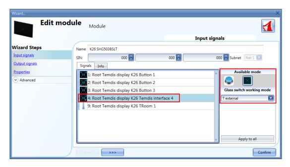
To see an external temperature, the user has to configure a key as *temdis interface* and then select *T external* in *Glass switch working mode*.
