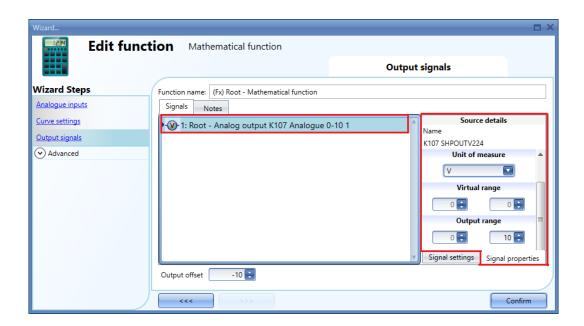
If the minimum and maximum virtual values of the function are 0 and 100, and the virtual output value is 30, the voltage output of the SHPOUTV224 will be 3V
