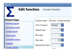
If the max and min values of the counting function are 100 and 0, and the virtual output value is 30, the voltage output of the SHPOUTV224 will be 3V.
