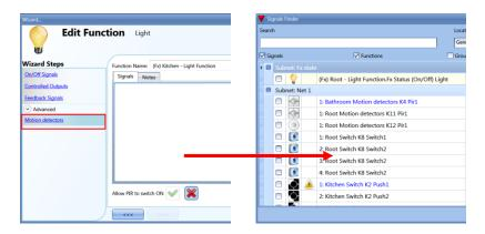
4. Enable it to switch the light ON
