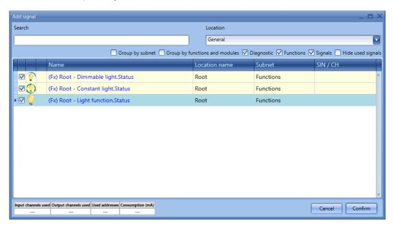
The functions available in this window are Light On/Off, Dimmable light and Constant light functions. Up to 100 functions can be chosen and they are managed in parallel.
