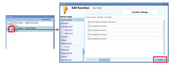
3. Click on the *Confirm* button to refresh the *Smart light* function, then click on the *Send to controller* button to download the configuration to the UWP 3.0 controller.
