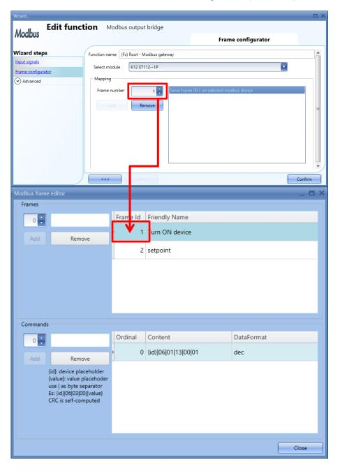
As a result of this configuration, each time the pushbutton is pressed, the Modbus RTU command *Turn ON device* will be sent to the Modbus device selected in the *Modbus output bridge* function.
