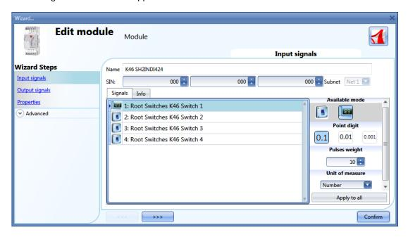
As for the settings of the SH2INDI424, the user has to select the working mode: it might be configured as a switch (the switch icon has to be selected), as a pulse counter by selecting the icon with 123, or as a push button. With this configuration the weight of each pulse can also be set in the *Pulse weight* field.
