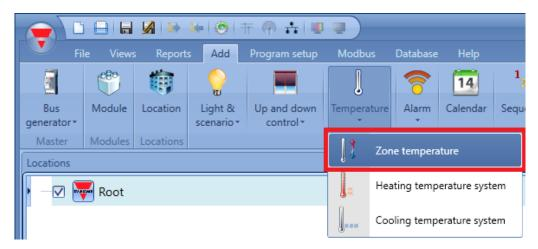
The last step is to link the temperature system function to the zone temperature functions: to do this the user has to open the zone function, click on *System temperature function*, double click on the correct window (according to the heating or cooling mode), and then select the required system function from the list of available functions (see picture below). More than one zone function can be controlled by the same system function.
