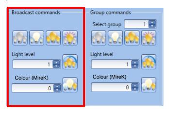
The broadcast commands can be executed to determine whether communication is working properly in the DALI circuit and whether all the devices in the DALI circuit are connected.
