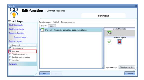
All the added functions will trigger the sequence according to the status they have: for example, a light that is switched on will make the sequence start; the same function that is switched off will make the sequence stop.
