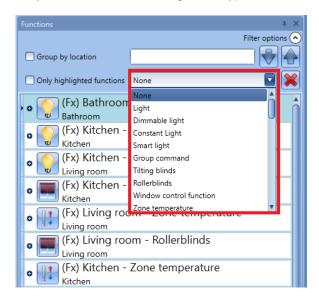
The user can remove the filters applied by clicking the red *X* icon.
