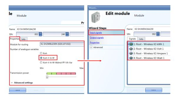
If the kWh-V-A-W-Wdmd-PF-VA-Var icon is selected by the user, the module will transmit all the variables related to this group: in the *Input signals* window a dynamic list shows all the analogue variables related to the group selected, as shown in the picture below.
