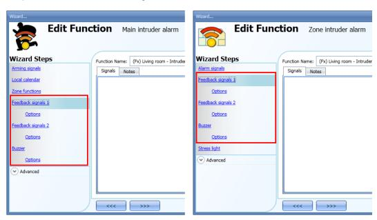
Regardless of the selected section (Feedback signal 1, Feedback signal 2 and Buzzer), the user can add LEDs, Relays and buzzers.
