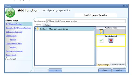
The inverted logic can be selected in the *Signal settings* tab window, as shown in the yellow rectangle above.
