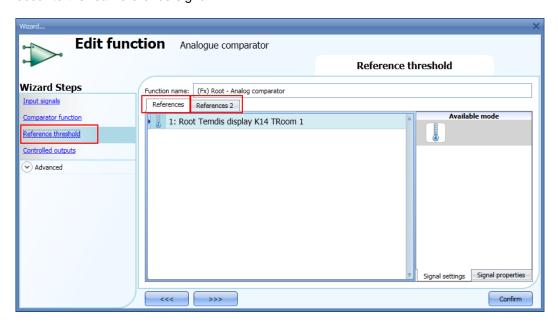
In the case of a comparator function with two reference signals (*inside limit* or *outside limit* type), Reference 2 is always used as the high threshold limit; Reference 1 is always used as the low threshold limit
