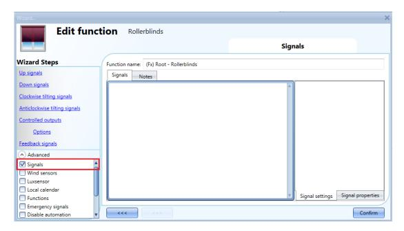
To add the signal to control the Up/Down movement and the tilting, the user should click on the relevant section, then double click on the *Signal* window and select the input signal from the list.
