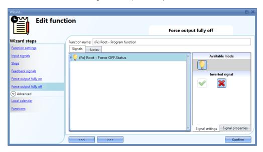
Each signal used in the *Force output fully off* window works in level mode. While the *signal* is active, the sequence is maintained inactive: all the Switch functions that belong to the steps will be maintained OFF and cannot be activated until the stop signal disappears.
