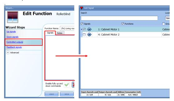
The signals available in this window are only the motor output type.
