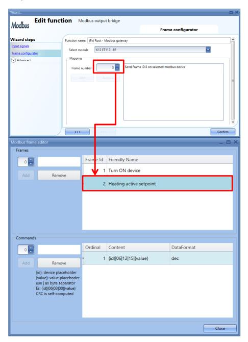
As shown above, the *Heating active setpoint command* **{id}|06|12|15|{value}** will be sent to the Modbus serial device every time its values change: as a result of this automation, the holding register indicated in the Modbus RTU command will be written with the new value.
