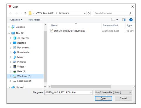
After having selected the correct file, the UWP 3.0 Tool automatically starts updating the UWP 3.0: once this operation is finished, the UWP 3.0 is automatically rebooted.
