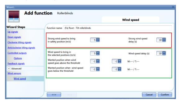
Highlighted in red: the user can select a strong wind threshold value - when the wind speed goes over this threshold, the blinds are automatically brought into the safety position (the safety position is fully up/down according to the settings in the output of the function).
