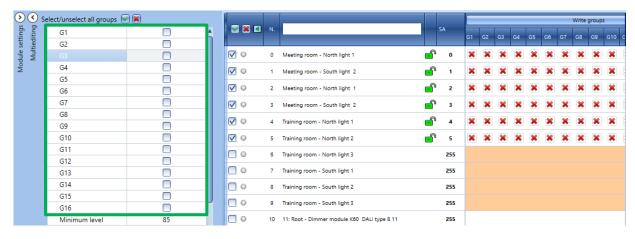
When the user clicks on a checkbox, (G1...G16), that Group will be applied to all the DALI ballasts selected in the Device list. As shown in the example below, the DALI ballasts 1 to 7 have been added to DALI GROUP 3 (G3 check-box). The user can check the group assignment in the *Device list* section (see the *green V* icons).
