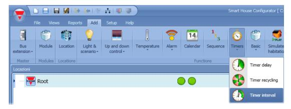
Using the interval timer, the output is activated by the trigger signal for a configurable interval time. The output of the timer is activated when one of the following events happens:
