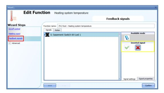
The inverted logic for the feedback can be selected as shown in the yellow rectangle in the picture above.
