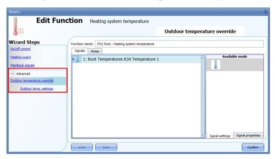
Firstly, the user should enter one or more temperature values coming from the temperature sensors. The user can add up to ten different temperature signals; if more values are linked, the average value is used. If a temperature sensor is faulty, the average value is calculated by using the other signals. In the field *Outdoor temperature settings*, the user can configure all the settings (see picture below).
