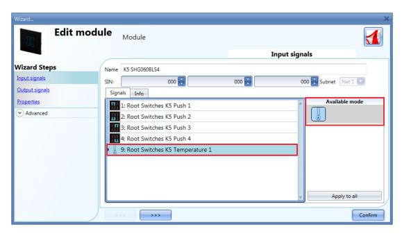
The SHG060WLS4 and SHG060BLS4 are glass switches with temperature sensors that can be used in any temperature function.
