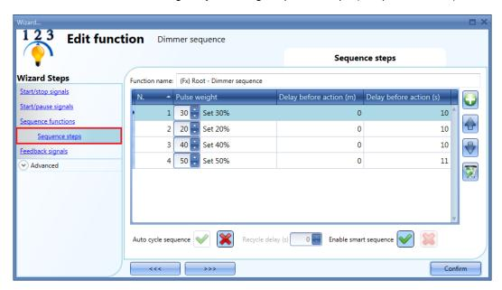
Auto cycle sequence: if this option is enabled, the sequence is repeated continuously: each time the last function is executed, the sequence starts again from the beginning. All the functions are
