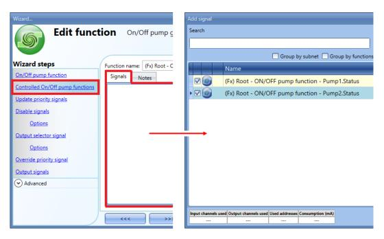
Up to 50 On/Off pump functions can be selected for each On/Off pump group function.
