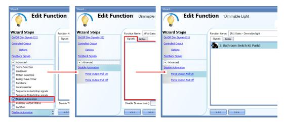
Each signal used in the "Force output fully on" window works in level mode. Until the signal is active, the light is forced to the fully on status. When the signal is non-active, the light returns to the previous status. When the *force to fully on* signal is activated and at the same time the *force fully off* signal is activated, the *force to on* status has priority.
