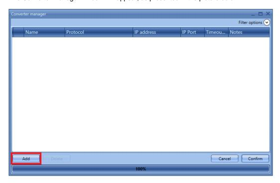
To configure a Modbus converter device, the user has to click on *Add* and then fill in the necessary settings:
