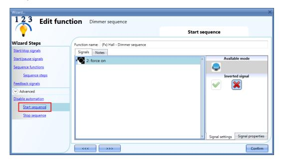
Each signal used in the *Start sequence* window works in level mode. While the start signal is active, the function is operative and cannot be deactivated until the start signal disappears.
