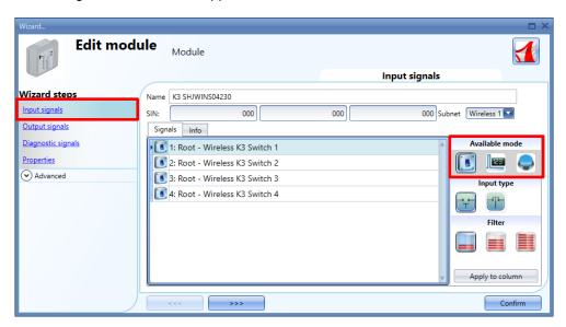
As for the settings of the SHJWINS04xxx, in the *Input signals* field the user has to select the working mode: this can be configured as a switch (the switch icon has to be selected), as a pulse counter by selecting the icon with 123, or as a push button (the third icon has to be selected).
