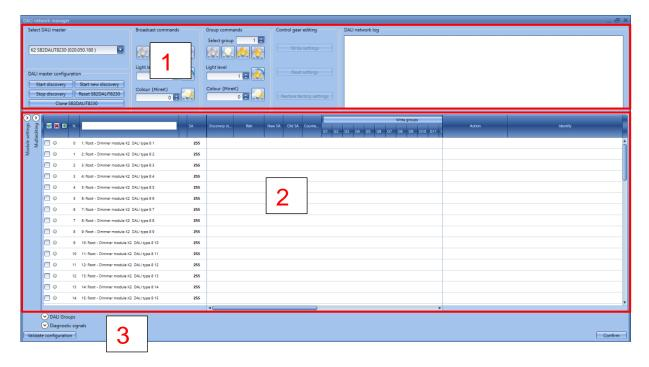
The DALI network manager window helps the user to configure, test and set parameters for DALI ballasts. It can also be used for grouping DALI ballasts and performing broadcast commands and group commands. The window is divided into three areas:
