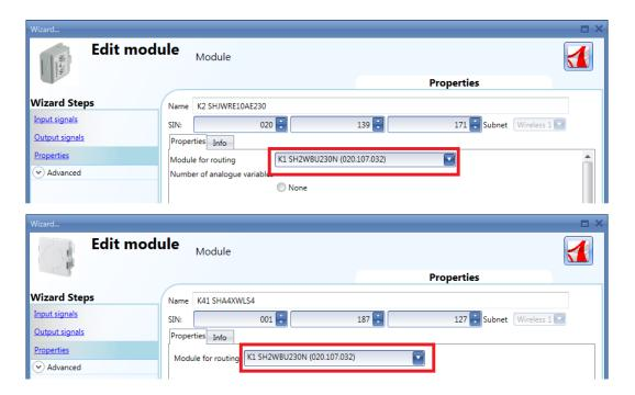
The picture below shows an example of a direct connection of two modules to the wireless base unit SH2WBU230x.
