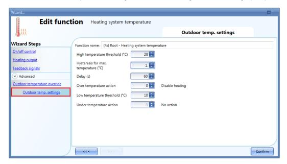
The user can set two different thresholds: the *High temperature threshold* and the *Low temperature threshold*.
