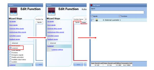
The user can add up to 10 lux sensors: if more lux signals are linked to the function, the average value is calculated and used.
