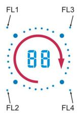
In the *Output signals* window, all the available feedback LEDs are shown and they can be used in the corresponding *Feedback* field of any function.
