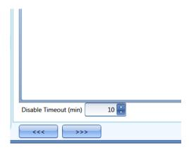
In figure above, a disable timeout of 10 minutes is set. The maximum delay is 59minutes.
