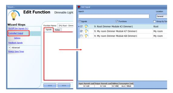
The signals available in the output window are only Dimmer output type.
