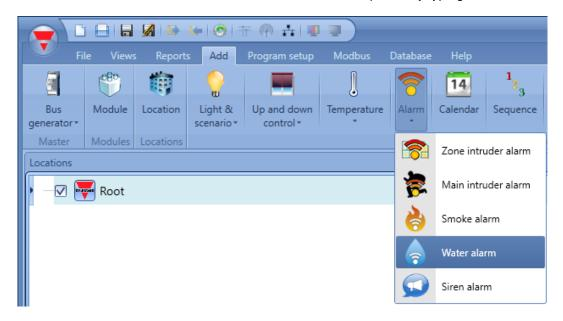
This function manages one or more outputs controlled by one or more input commands. The command might be a signal from a water detector, a pushbutton, a switch, a function or a remote command (Webserver, sms, Modbus TCP/IP)
