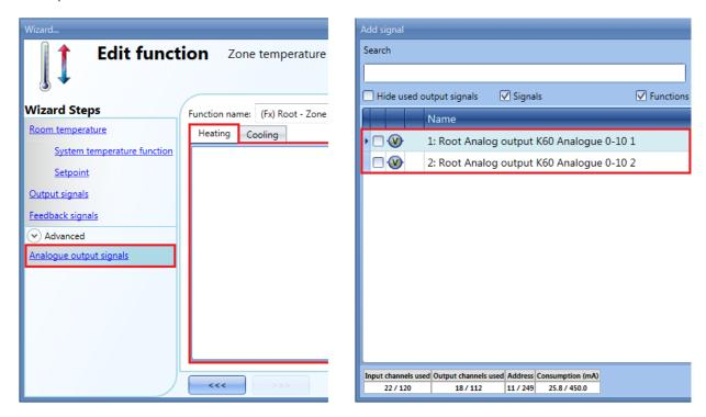
The output types available for this field are those from the module SHPOUTV224 (to control actuators with 0...10 V inputs).
