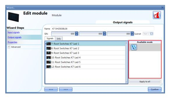
In the *Output signals* window, all the available feedback LEDs are shown: they can be freely programmed as feedback status LEDs for any smart-house function.
