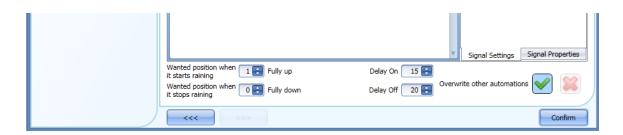
If the option *Overwrite other automations* is selected, until the rain signal is high, the other automations are disabled.
