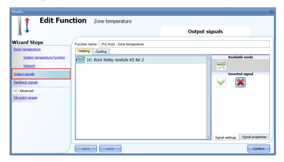
The on/off switching of the output is managed by the system temperature function according to the timing described in the paragraph *How to add the heating output*.
