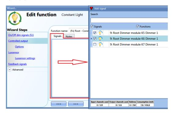
The signals available in the output window are only Dimmer output type.
