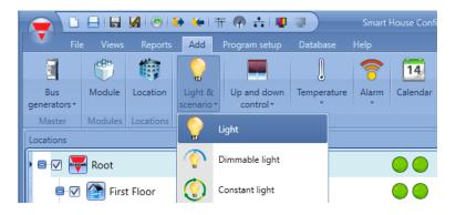
This function manages the ON/OFF switching of one or more outputs by means of one or more input commands. The input command might be a real signal, a function or a remote command (Webserver, sms, email, Modbus TCP/IP).
