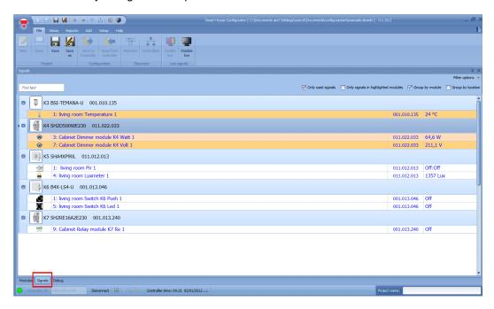
The second way is to click on the function where the signal is used and select *Used signals* in order to have a global view of all the signals used in the function.
