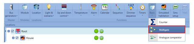
The multigate function can be used to perform different actions: for example to collect signals from more than one point to monitor, for example, door contacts or window switches in an alarm function, or to monitor more signals and/or functions to get a quick overview of a status.
