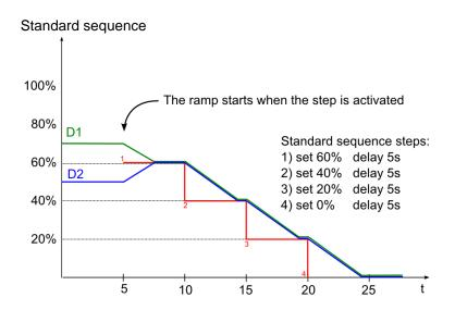
The following figure shows the behaviour of the dimmer sequence using the same steps.
