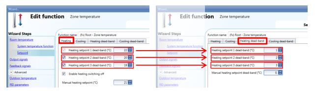
In the example shown above, setpoint1 is 21° (22-1) so heating will be switched off at 21° and switched on according to the set hysteresis; setpoint2 is 18° (20-2) so heating will be switched off at 18° and switched on according to the set hysteresis; setpoint3 is 15° (18-3) so heating will be switched off at 15° and switched on according to the set hysteresis.
