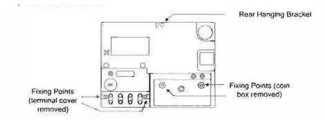
When installing the meter, initially it should be hung from the rear hanging bracket using a suitable round headed screw. The screw depth should be adjusted so the head fits snugly under the hanging point and the meter is held firm against the wall. Once hung, ensure the meter is level then mark and screw the meter to the wall securely using the four fixing points; two are located under the grey terminal cover and two are under the coin box (see drawing above).
