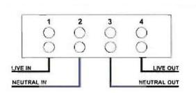
The meter must be protected against overcurrent. This is normal as part of the building installation (Service fuse to 6S1361) or equivalent; maximum current through the meter must not exceed 100 Amps.
