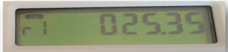
In this example the rate is set to 25.35 pence per unit. If you are using a 2 rate tariff system, rate 2 will be displayed by pressing the Display Cycle button once more until 'r2' is indicated
