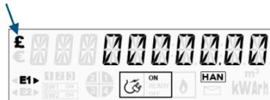
Displays with text on the right-hand side will use a hyphen ('-') as a decimal point. For example, the numeric display in the following example should be read as '000.000 pence'.
