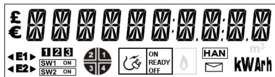
Figure 8: Meter display in 'Test Mode'
