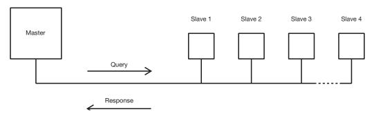
In the MODBUS Protocol the master can address individual slaves, or, using a special "Broadcast" address, can initiate a broadcast message to all slaves. The SDM630 Digital meter do not support the broadcast address.
