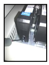
**3** - Clip the top of the new Comms module onto the din-rail and using the flat screw driver to open the din-rail release clip, while pressing the module fully down on the din-rail.
