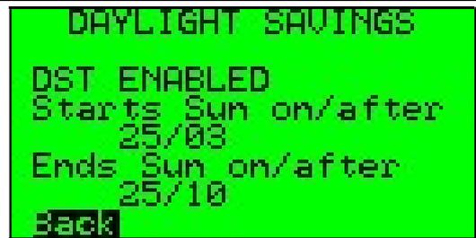
**Note:** Setting the dates for Daylight Savings does not affect the real time clock or the data logger operation. The daylight savings setting merely allows Day Data files, stored in the logger, to include a flag on days when daylight saving should be applied in external systems.
