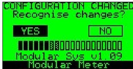
The detected modules are recognised and shown in their position and the user is requested to accept these changes.
