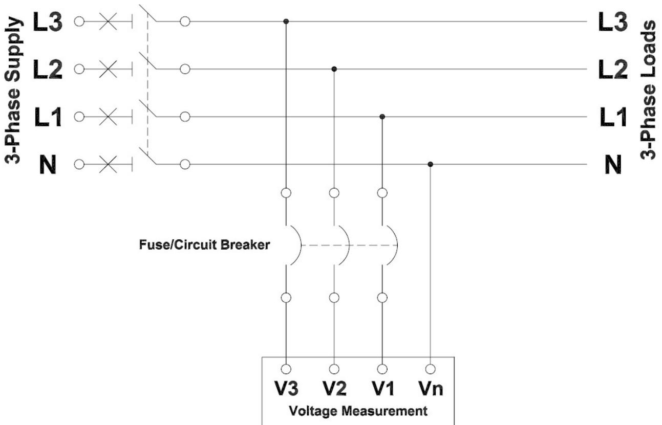
**Figure 4-2 Measurement Voltage Inputs**
