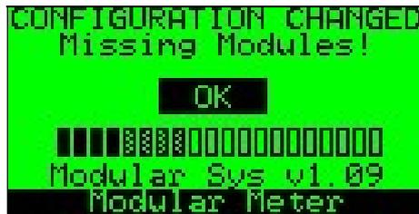
**NOTE:** The "Configuration Changed" screen times out after approximately 30 seconds.
