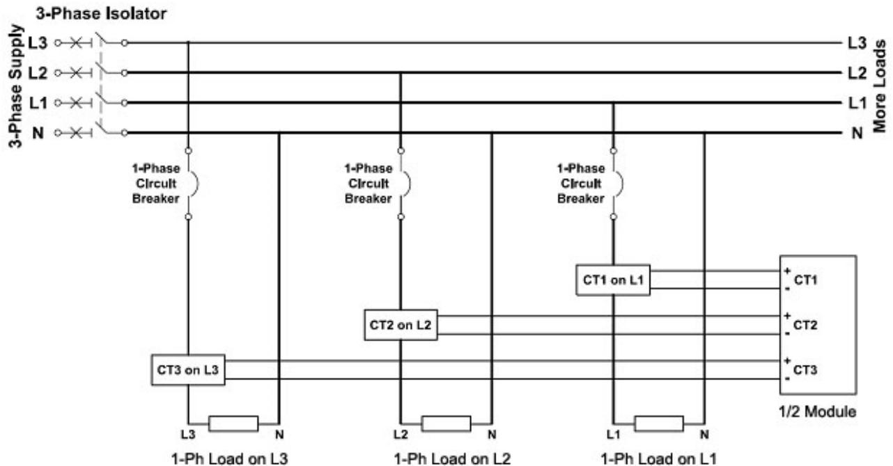
Figure 4-4 Measuring 3 x Single Phase Loads Using 1/2 MC352
