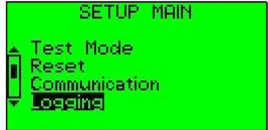
**NOTE:** New meters are supplied with logging STOPPED. Only when the logger is STOPPED can a new session can be setup or major changes made to the logger configuration. This prevents corruption of the data format in during an ongoing log session.
