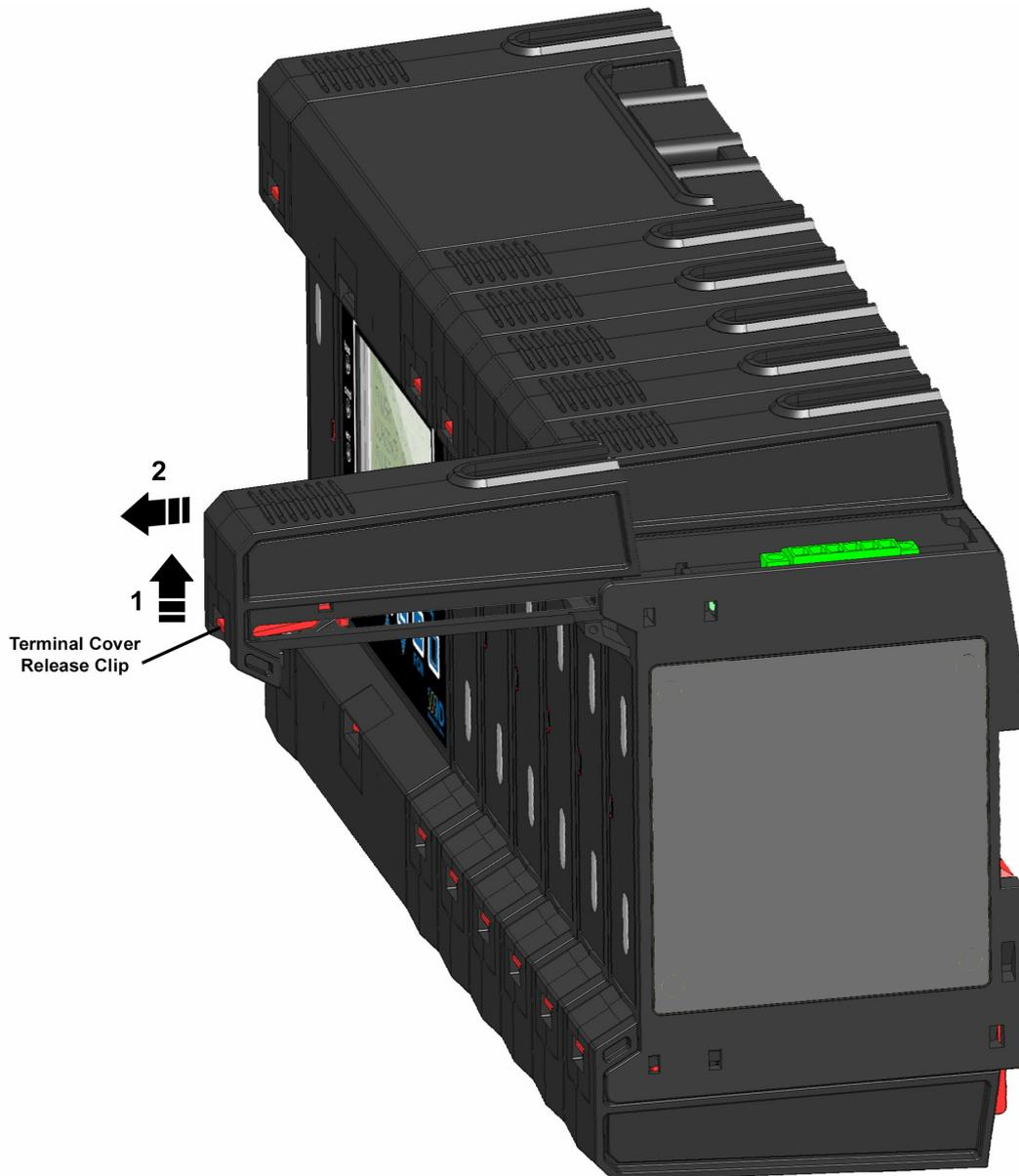
**NOTE:** The release clip may be covered with a tamper evident label (20mm x 18mm) to detect unauthorized access.
