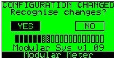
The detected module(s) are recognised and shown in their position and the user is requested to accept the changes.
