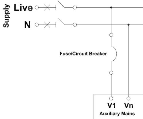
**Figure 4-1 Auxiliary Mains Connection**
