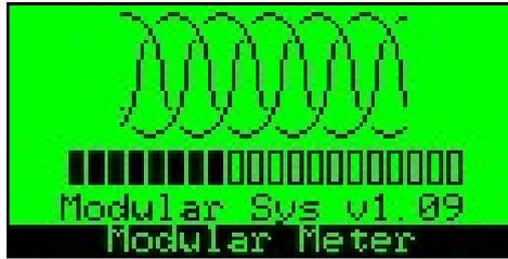
The power up screen details the software version for the Master Display Unit and a progress bar shows connection of each Sub Module as it is automatically identified. This screen is displayed for approximately 10 seconds.
