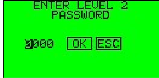
**NOTE:** If a password of 0000 is set, the password entry screen is not shown and immediate access is granted.
