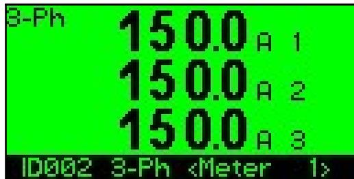
This page shows measured values from the selected meter/load. This data is meaningless for an unconfigured **multicube** system as the programmed Current Transducers may not match the physical devices fitted.
