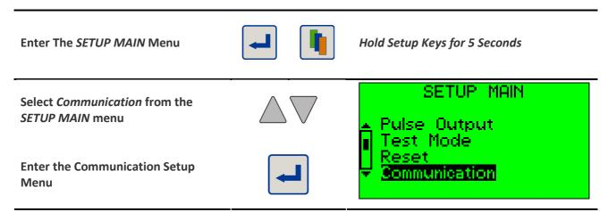
When the **multicube** has correctly identified that a TCP/IP Ethernet interface module is attached (during power up) the menu options in the Communications Menu are changed to reflect the different settings required.
