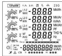
The first screen lights up all display segments and can be used as a display check.
