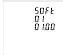
The second screen indicates the firmware installed in the unit and its build number.
