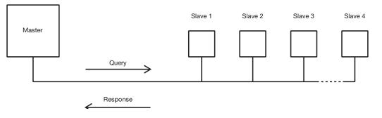
In the MODBUS Protocol the master can address individual slaves, or, using a special "Broadcast" address, can initiate a broadcast message to all slaves. The SMARTRAIL X835 Digital meter do not support the broadcast address.
