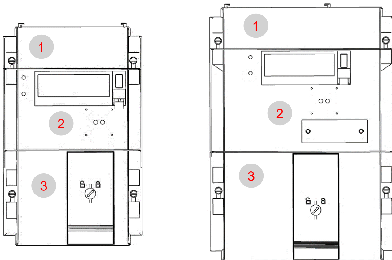
Figure 23: The main meter parts of the single-phase (left) and three-phase meter (right)
