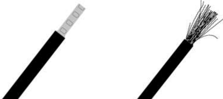
Figure 49: Properly prepared cables
