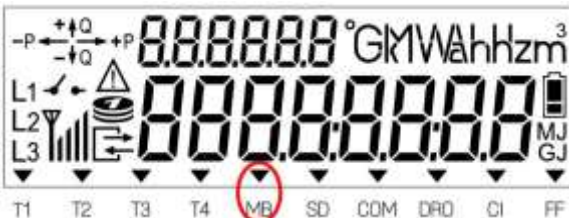
Figure 122: M-Bus display cursor
