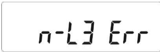
Figure 73: Example of wrong Neutral-Phase connection indication text on display
