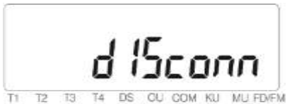
Figure 107: dISconn on the display
